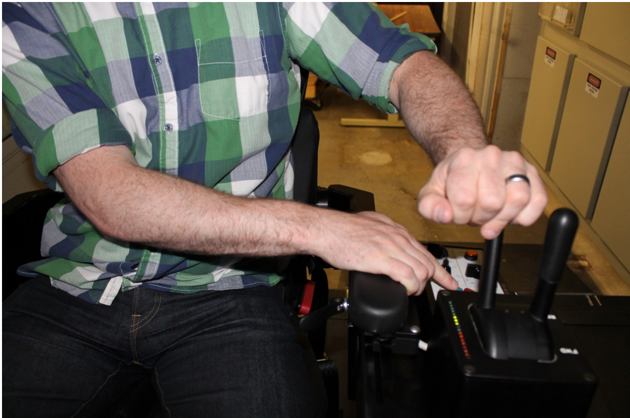
Figure 41. Two-handed operation for simultaneous use of the horn and throttle
