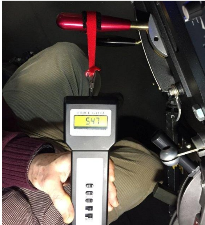
Figure 19. An evaluator using the handheld force gauge to measure the automatic brake in AAR-105 control stand in CTIL
