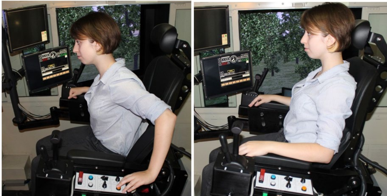
Figure 13. Posture required to actuate the alerter on the experimental crewstation (left), and natural hand position (right)
