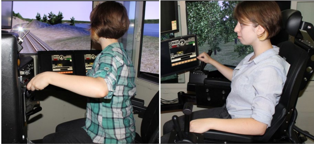
Figure 21. A 50 th percentile female evaluator operating the automatic brake in the AAR-105 control stand in CTIL (left), and the experimental crewstation (right)
