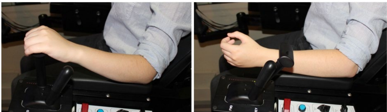
Figure 24. Use of experimental crewstation levers with limited forearm support (left), suggested position of levers to improve utilization of armrests (right)
