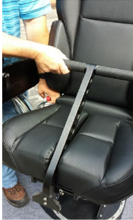
Figure 14. Experimental crewstation seat conversion step showing engineer holding the footrest (right hand) while pulling the seat pan's drop lever (QNA Transportation Group, 2014)
