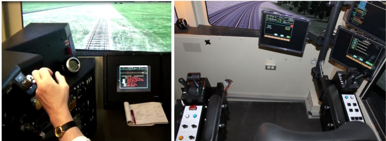
Figure 12. Engineer's view and workspace. AAR-105 control stand with desk space for worksheets (left), experimental crewstation without desk (right)
