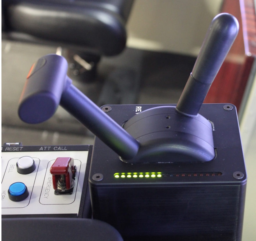
Figure 5. Combined dynamic brake and throttle on the experimental crewstation
