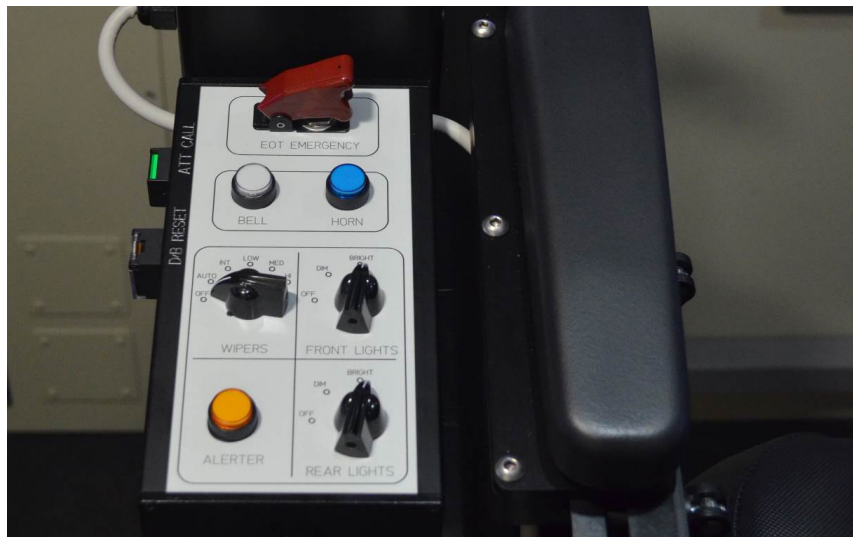
Figure 28. Left armrest control box with labels written in black text on a light gray background
