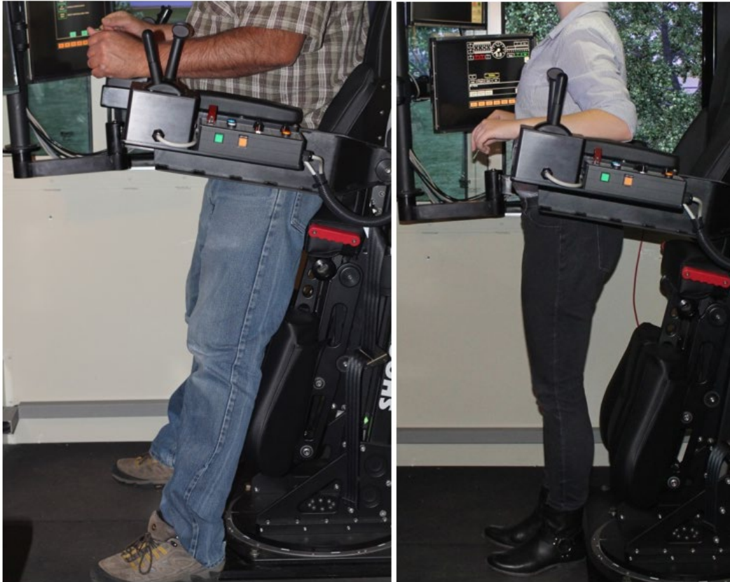
Figure 27. An approximately 95 th percentile male (left) and 50 th percentile female (right) during standing operation demonstrate the lack of armrest adjustability
