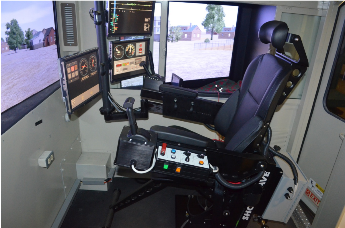
Figure 4. Experimental crewstation with integrated controls and displays
