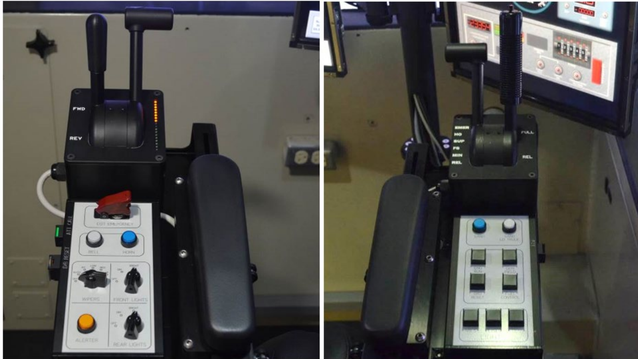
Figure 23. Left hand side controls including throttle and dynamic brake, reverser, end-of-train emergency switch, horn, bell, lights, and alerter (left). Right hand side controls including automatic brake, independent brake, sand buttons, engine run, generator field, fuel control, grid reset, and lights (right)
