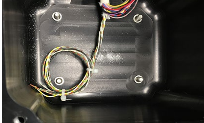
Figure 17. The silver powder-like crystals shown inside of the throttle control box are aluminum shavings from the detent housing caused by wear from the control lever's steel ball bearing
