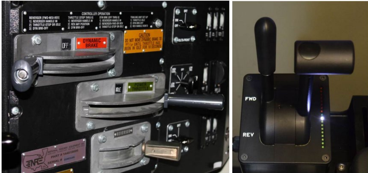
Figure 16. Dynamic brake and throttle levers on the AAR-105 control stand (left) and on the experimental crewstation (right)
