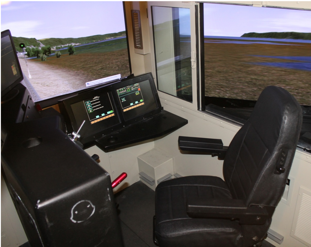
Figure 3. CTIL-provided seat angled toward the AAR-105 control stand in the simulator
