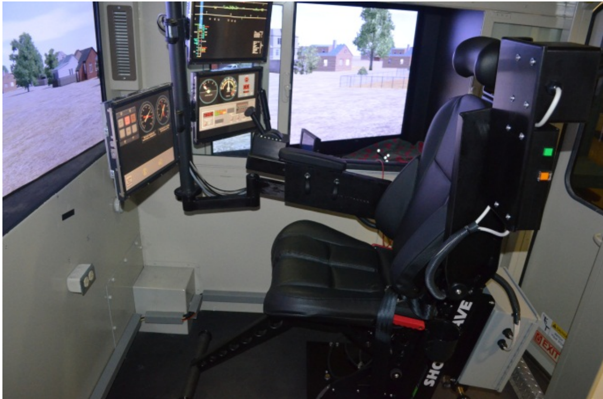
Figure 1. The experimental crewstation
