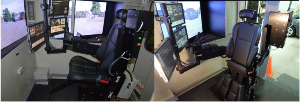
Figure 6. Experimental crewstation configured for seated operation (left) and standing operation (right)
