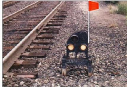
**Figure 23. Retroreflective Border and Marker on Signals**
