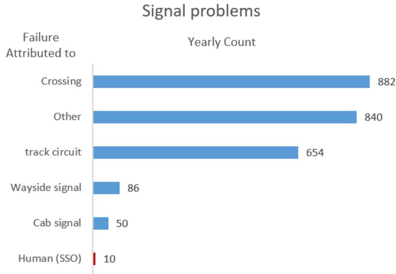
**Figure 15. Frequency of Signal Problems by Type**
