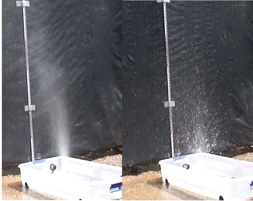
Figure 15. Left: Height of Spray from Single 1/8-in. Hole (~4-5-ft. tall); Right: Height of Spray from Single 1/4-in. Hole (~3-ft. tall)
