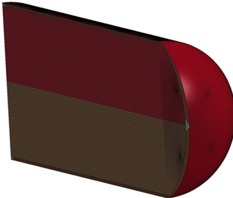
Figure 6. Quarter-Scale FE Model of Tank
