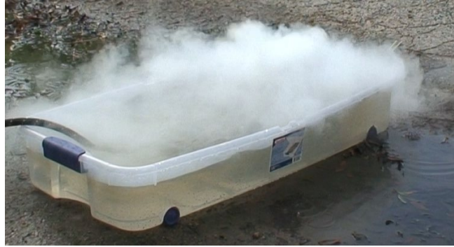
Figure 18. (3) × 1/8-in. Diameter Holes in 2-in. Diameter Pipe with 2-in. Wide Plate Cover, 1-in. Gap Between Steel Plate and Pipe Holes, 1.5 gpm
