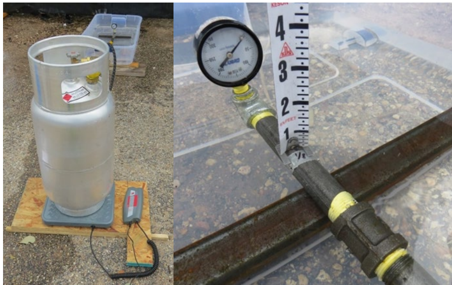
Figure 13. Small-Scale LPG Burner Test Setup
