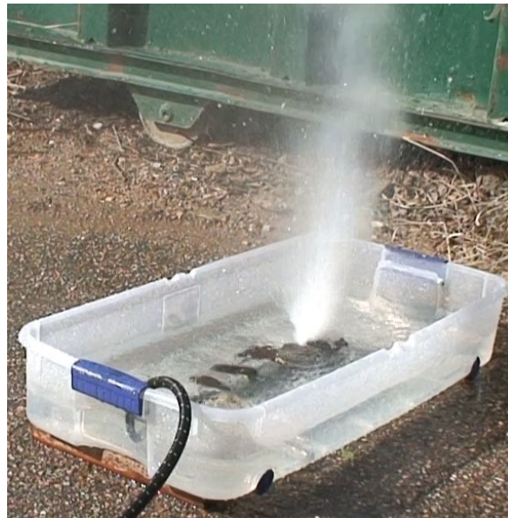
Figure 14. (3) × 1/8-in. Diameter Holes, 2-in. Diameter Pipe, 1.5 gpm
