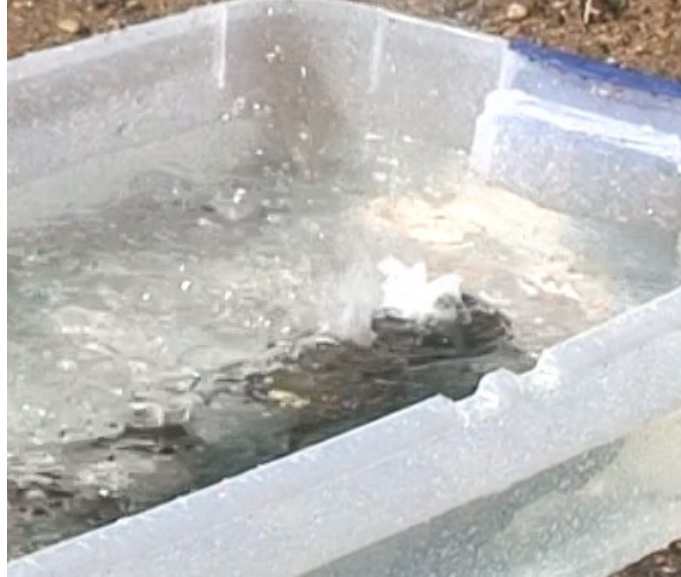
Figure 16. Ice Buildup: (2) × 1/4-in. Diameter Hole in 2-in. Diameter Pipe at 1.5 gpm
