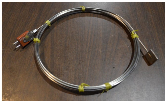
Figure 30. Weld-Pad Surface Temperature Thermocouple Probe
