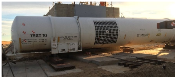
Figure 1. Pre-test Photo of DOT-113 Tank Car
