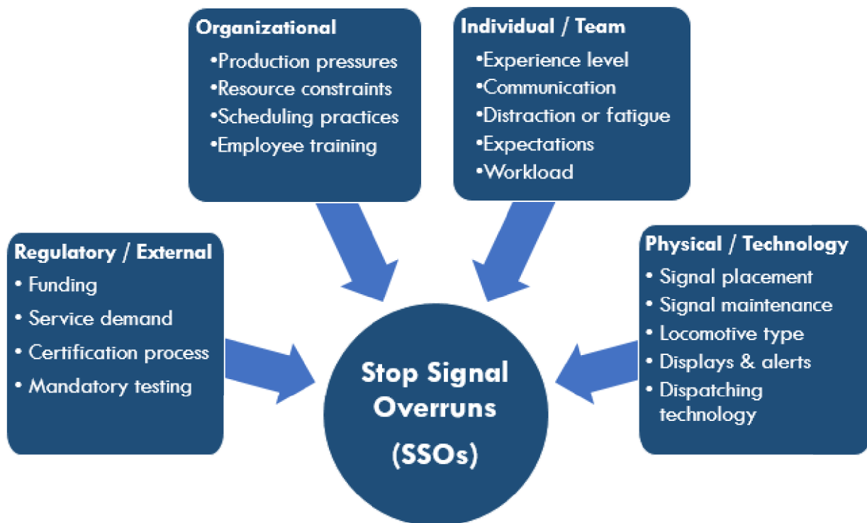
Figure 2. Factors that can combine and interact in different ways to exert a negative or positive effect on SSOs
