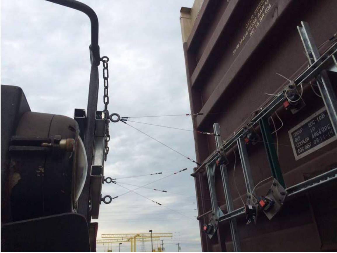
Figure 6. String potentiometers connected between locomotive and box car
