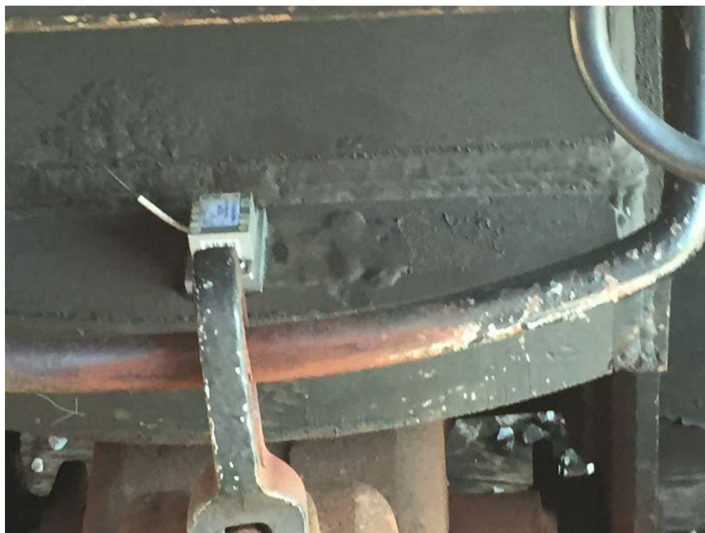
Figure 8. Accelerometer mounted on the locomotive end sill
