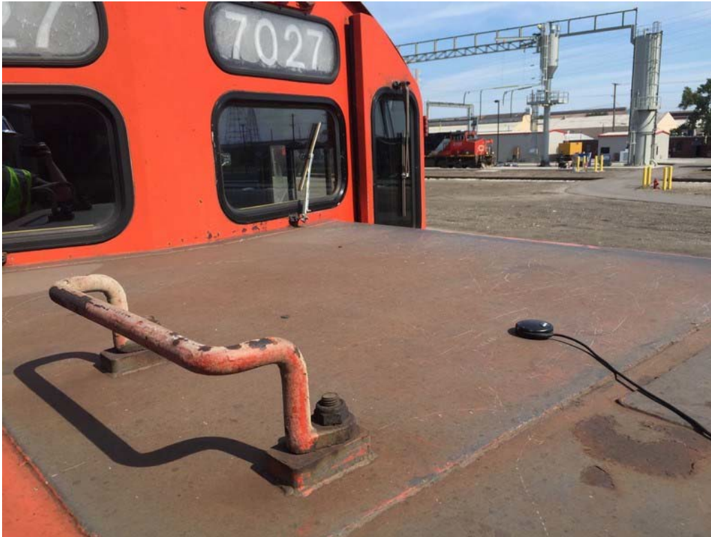
Figure 9. GPS antenna installed on locomotive short hood
