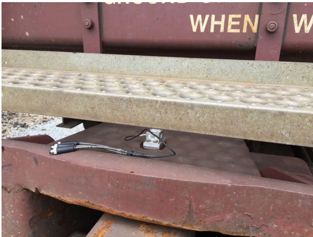
Figure 7. Triaxial accelerometer mounted on box car prior to testing
