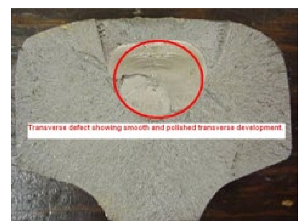
Rail Flaws to Image: Transverse Fissure
