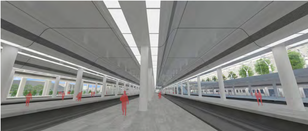
Figure 70. View from Stub End platform with deck level at 96' and soffit at 80' (24.5' clear at platform)
