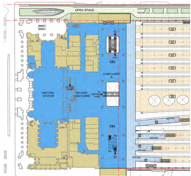
Figure 49. Bus on South: Partial Plan at Main Concourse Level (Bus Terminal Above)
