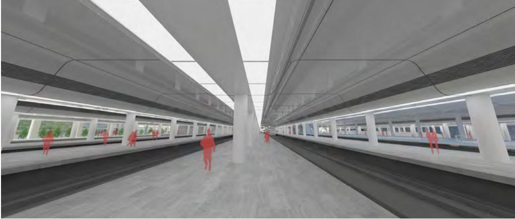
Figure 69. View from Stub End platform with deck level at 86.25' and soffit at 70.25' (14.5' clear at platform)
