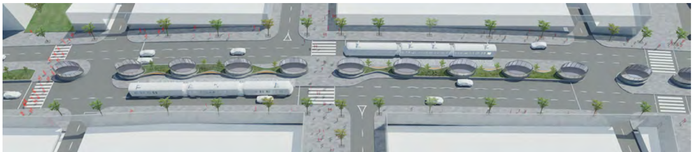
Figure 122. Overhead View of H Street Bridge with Integrated light-wells within the central median
