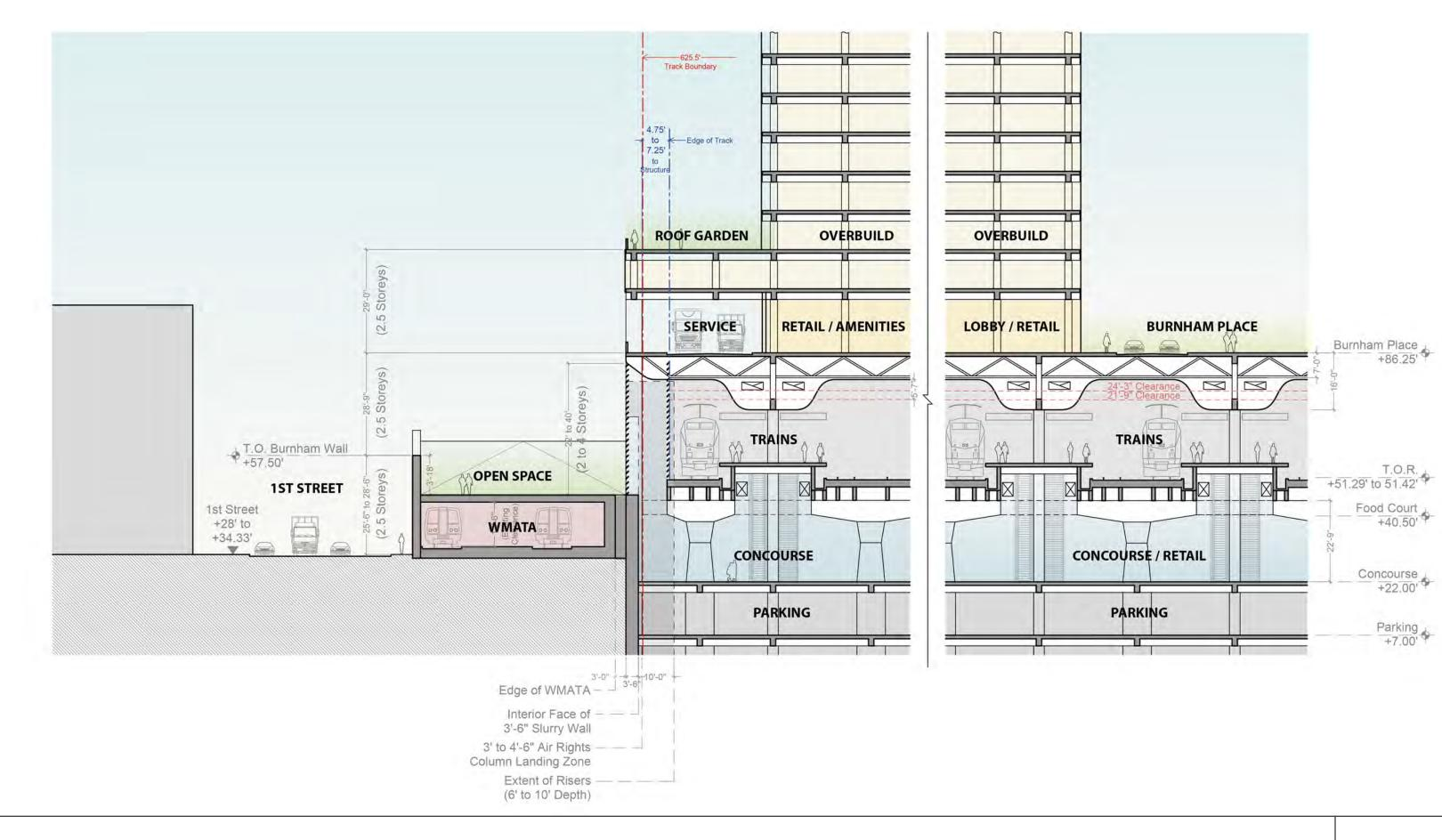
**EDGE SECTION** SOUTHWEST (BOTTOM OF OVERBUILD STRUCTURE AT +70')
