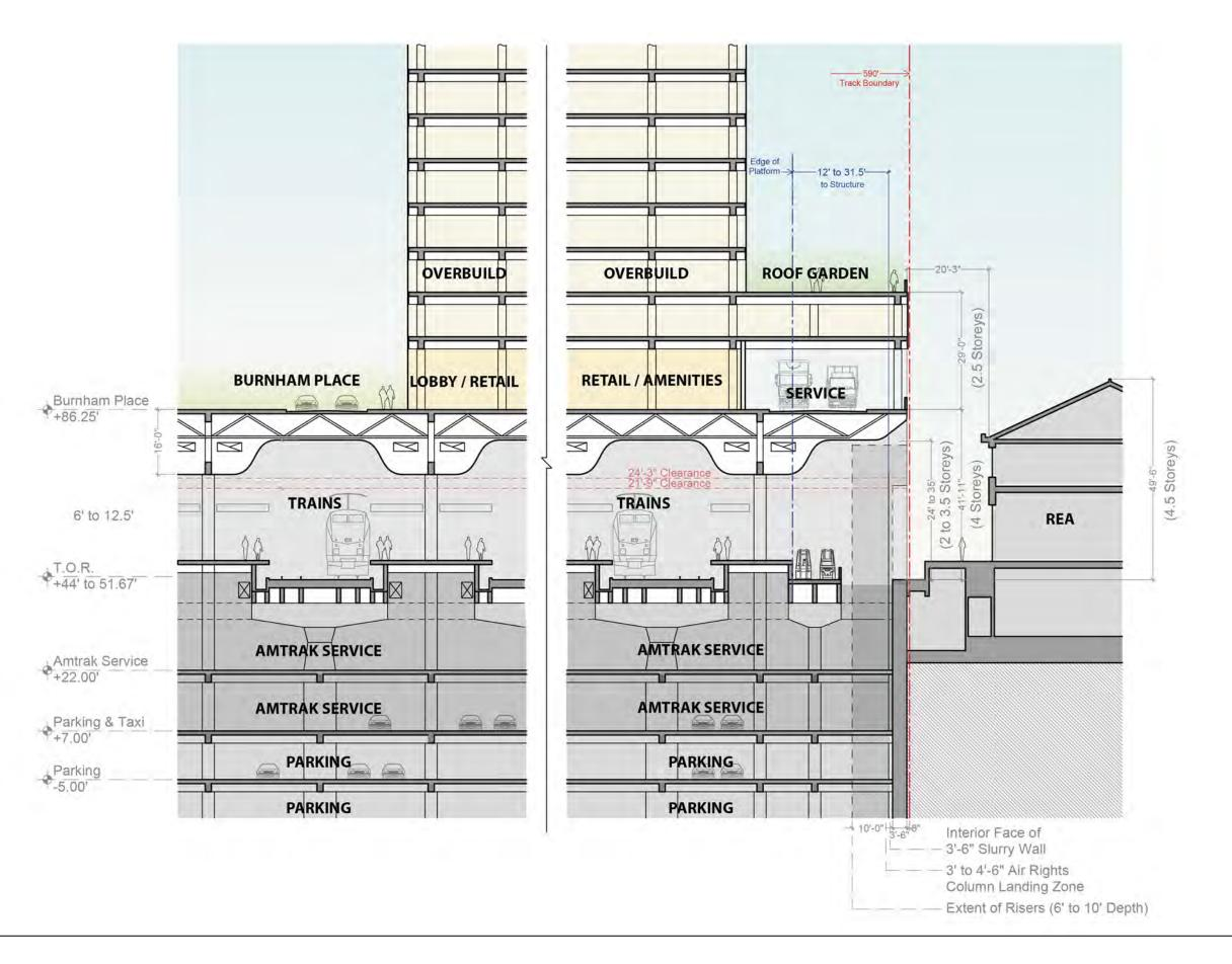
EDGE SECTION NORTHEAST (BOTTOM OF OVERBUILD STRUCTURE AT +70')
