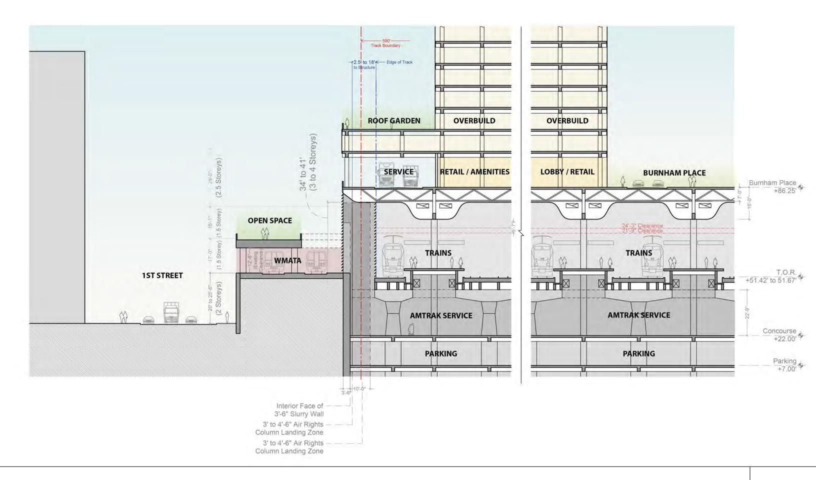
**EDGE SECTION** NORTHWEST (BOTTOM OF OVERBUILD STRUCTURE AT +80')
