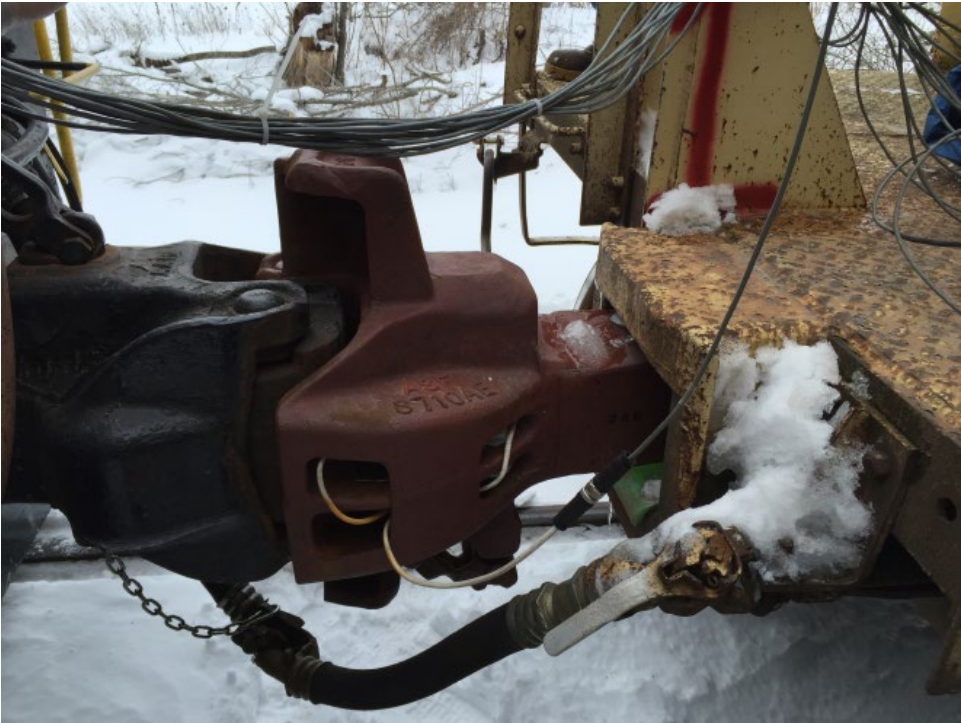
Figure 2-11. Dynamometer coupler installed in Test Car 1 (right)
