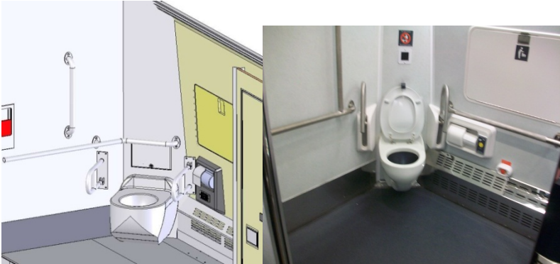
Figure A 11 Toilet with grab bars and fold away arm supports on each side of toilet, illustrating clear housing for frontal approaches (VIA Rail Canada)
