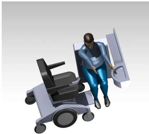
Figure 4-5 5th Percentile Female Manikin Evaluating Toilet-to-Sink Reach Range
