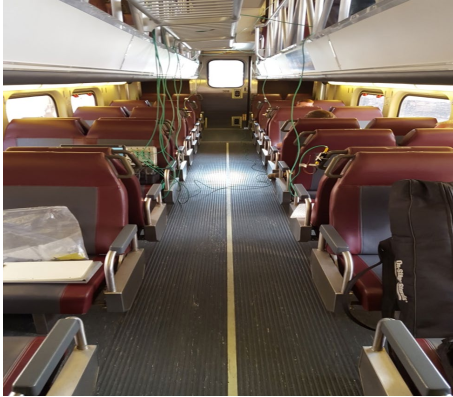
Figure 2-2. Instrumentation of the bi-level passenger coach
