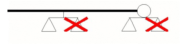
Partial Activation Failure; Full warning not given for each lane of approaching traffic.
