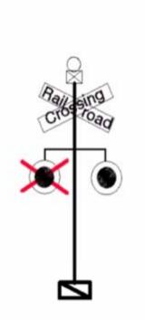
Partial Activation Failure, gate arm broken holding flashing marker light.
