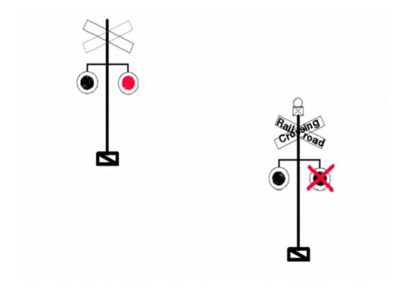
Partial Activation Failure, single pair of flashing lights on approach to crossing, no back lights visible.
