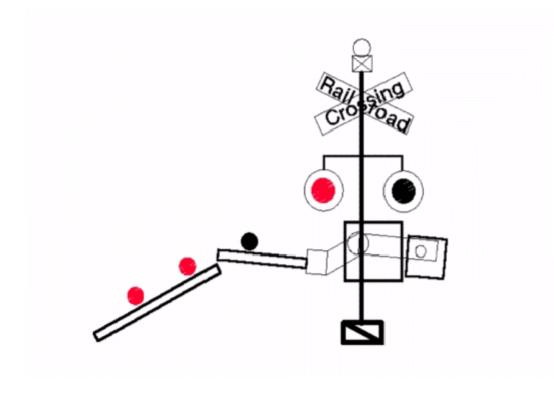
Track Speed; Gate arm tip broken outside of flashing gate lights.
