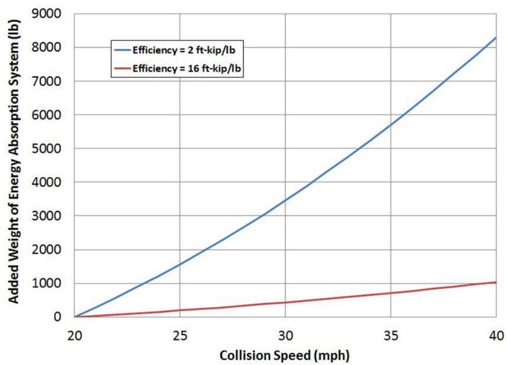
Figure 27. Additional weight required to achieve higher collision speeds in the Tier III train-to-train collision scenario; subject train weight is 950,000 lbs
