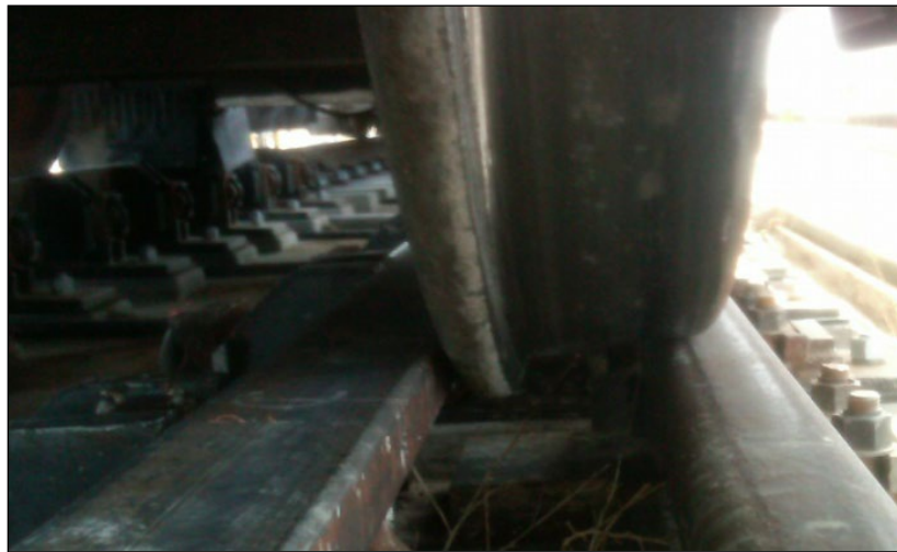
Figure 5. TLV Wheel on Trackwork (Back of Flange Spacing is Same on Other Side)
