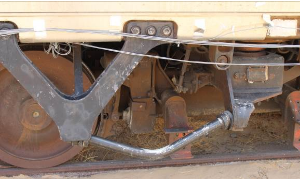
Figure 102. Bent Traction Rod after Sixth Test
