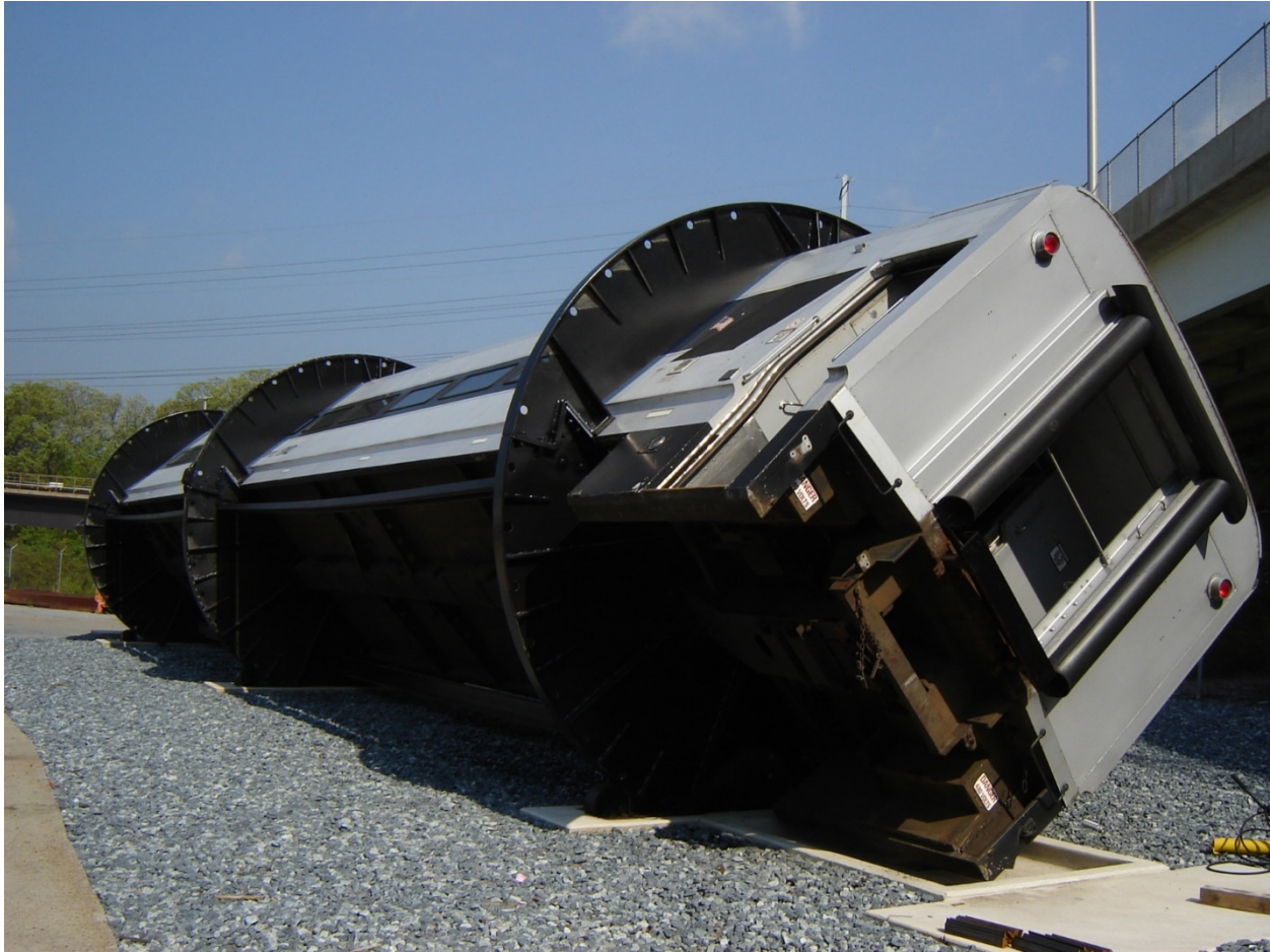
Figure 1. FRA-Sponsored Rollover Rig at WMATA Carmen E. Turner Training Center
