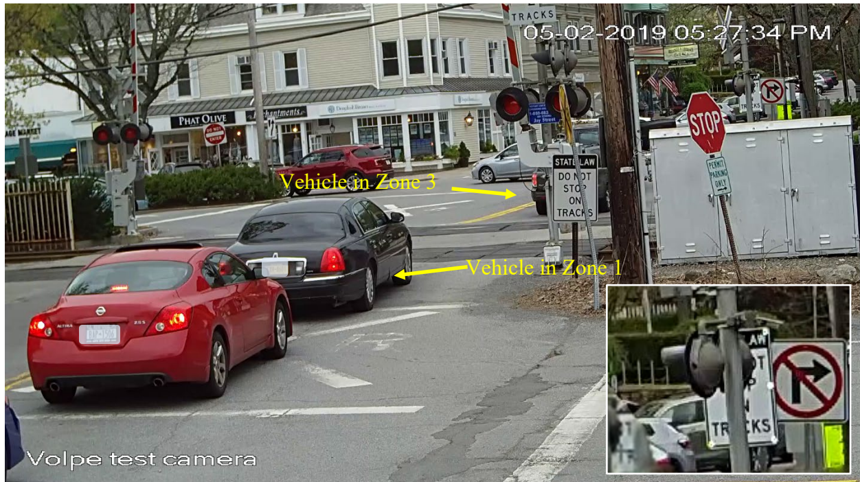
Figure 19. Vehicles queued on the westbound approach to Jay Street. Inset shows LED-enhanced NYR9-5 sign is activated.
