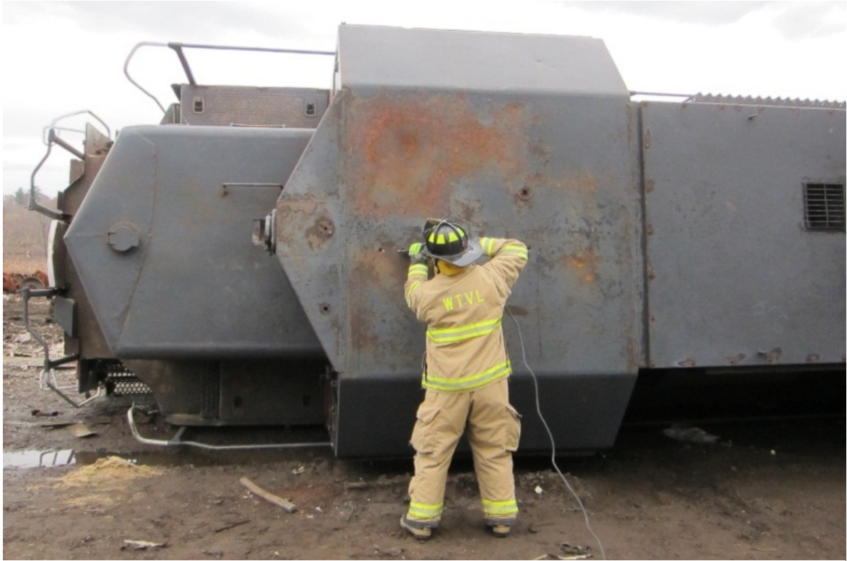
Figure 11: Cutting Opening into Roof Using Sawzall
