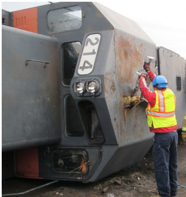
Figure 12: Using Hydraulic Spreader to Peel Back Roof
