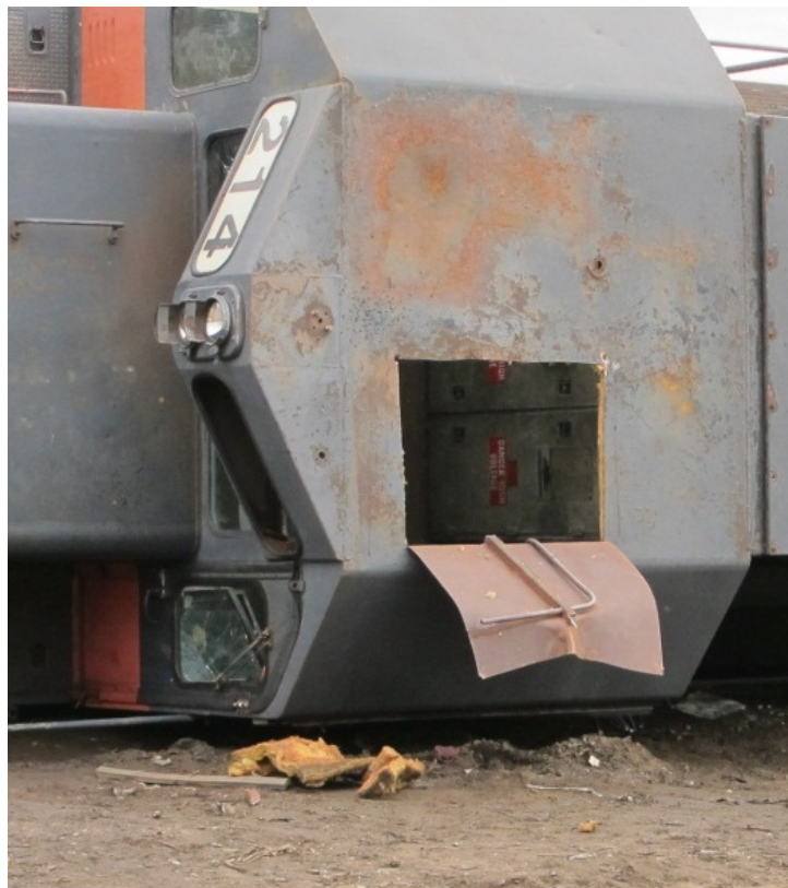
Figure 14: Final Roof Egress Point
