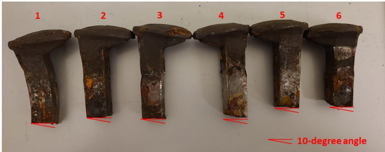
Figure 23. Orientation of cut spike failure plane
