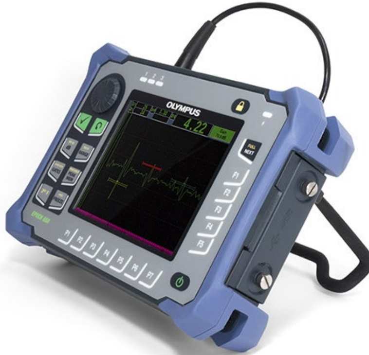
Figure 18. Ultrasonic flaw detector Photo credit: Olympus Corporation
