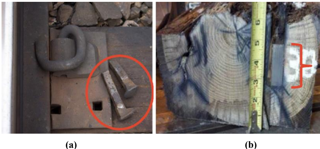
Figure 1. (a) Broken cut spikes and (b) broken cut spike within a wood crosstie [1]
