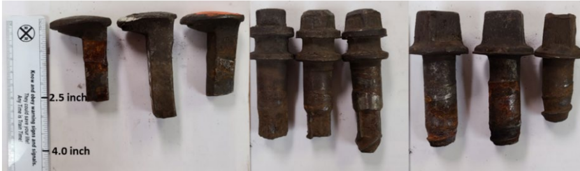
Figure B1. Failure plane locations on broken spikes of different spike types from FAST
