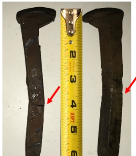
Figure B2. Failure plane locations on cut spikes (rail spike location) from revenue service
