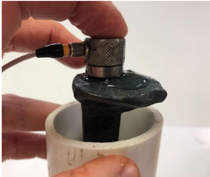
Figure 19. Transducer on a cut spike
