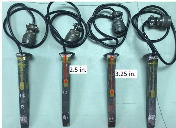
Figure 2. Instrumented locations of strain gages
