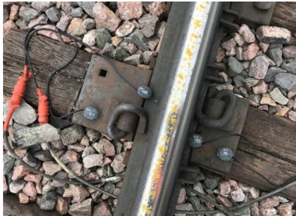
Figure 1. Instrumented spikes in a tie plate
