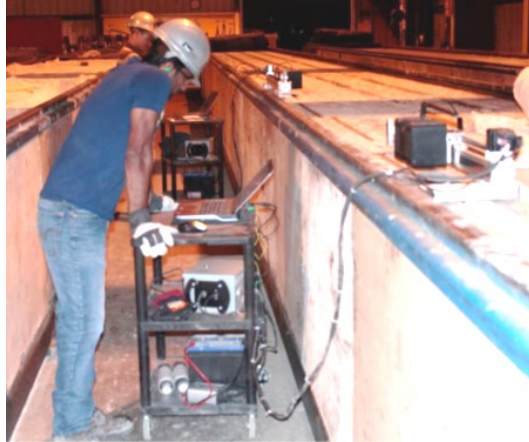
Figure 7: LSI surface-strain measurement system
