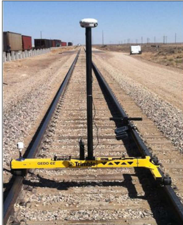
Figure 9. Survey Trolley with HA-GPS Installed
