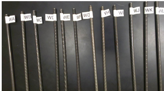
Figure 2: Researchers used 12 different 5.32-mm-diameter wires with unique indentation types
