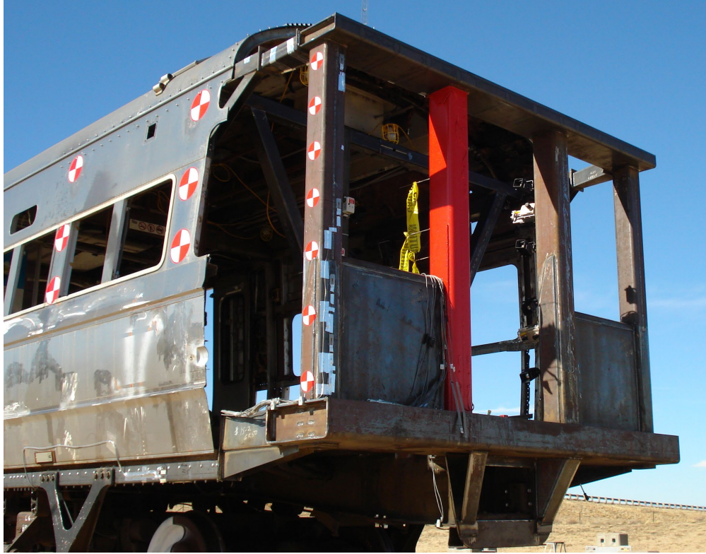
Figure 16. SOA end frame integrated with M1 car
