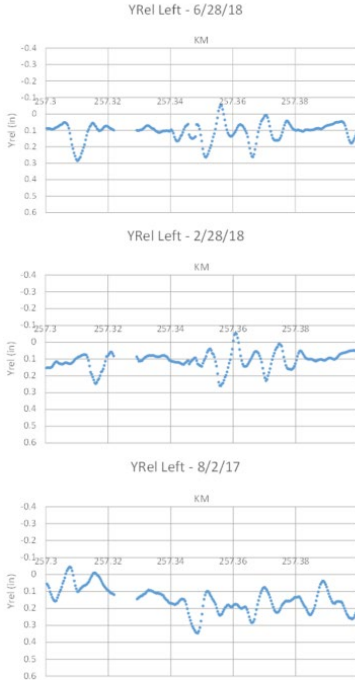
Figure 24. Mud spot approximately at KM 257.35 for multiple inspections
