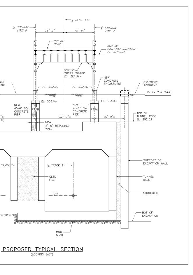
High Line Structure Underpinning — Existing and Proposed Typical Sections Figure D-2
