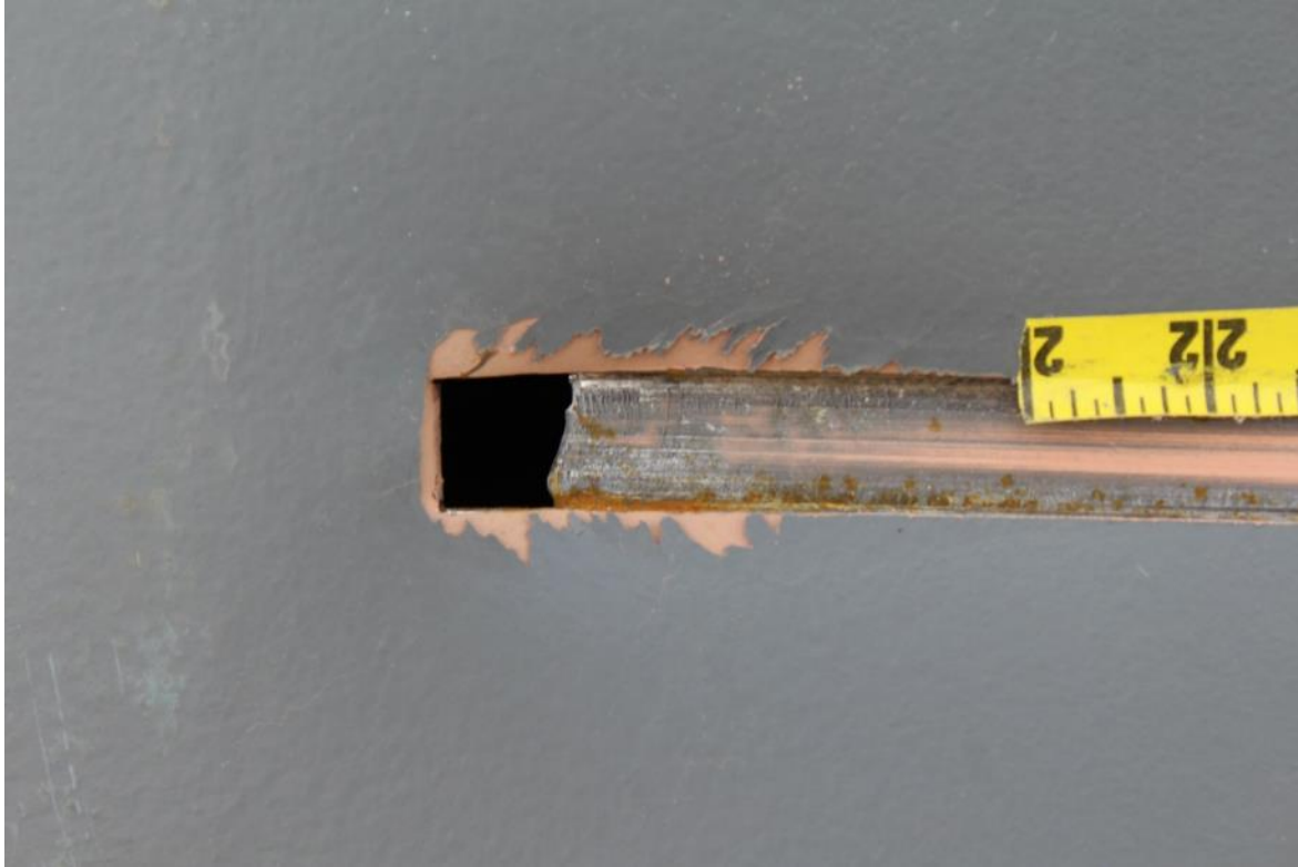
Figure 46. Second Tear in Test 2 Fuel Tank
