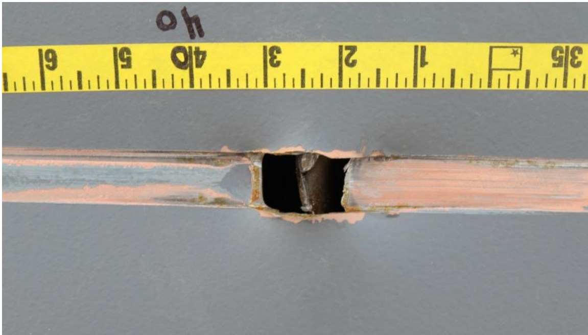
Figure 45. First Tear in Test 2 Fuel Tank
