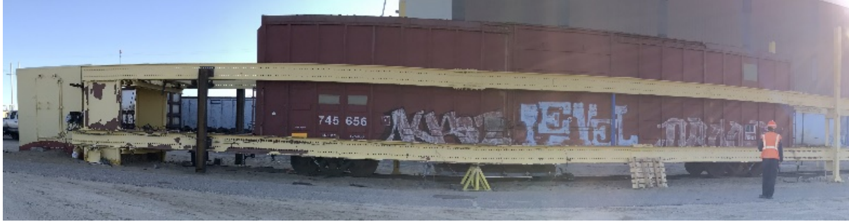
Figure 9. View of Boxcar in Test Fixture and View of Indenter Setup
