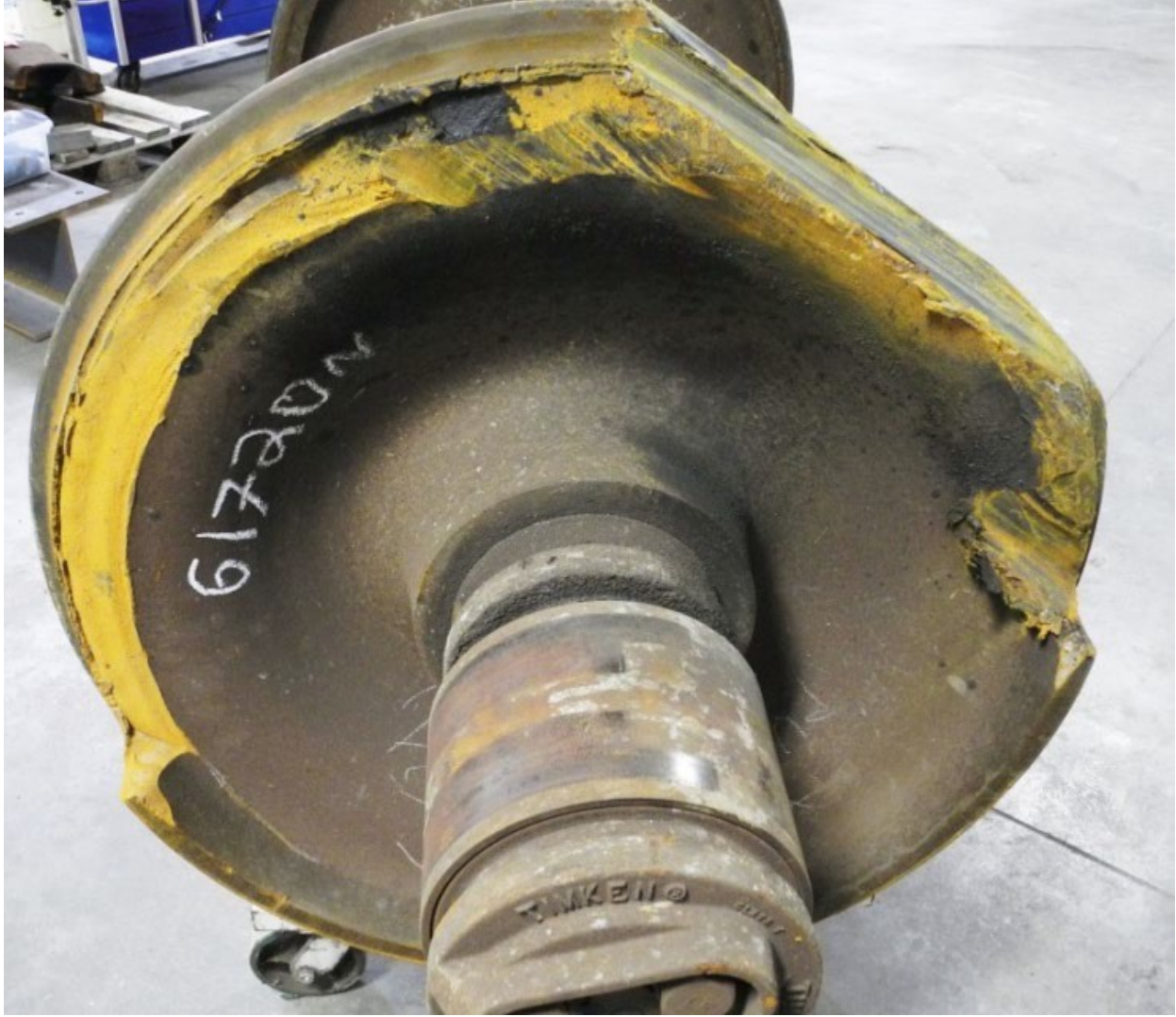
Figure A-41. Fractured Wheel CSX8, as Received
