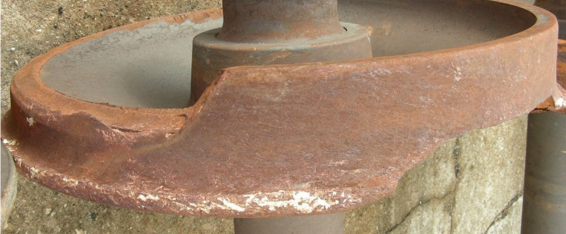
Figure A-18. Location of VSRs on Front and Rear Wheel BNSF3
