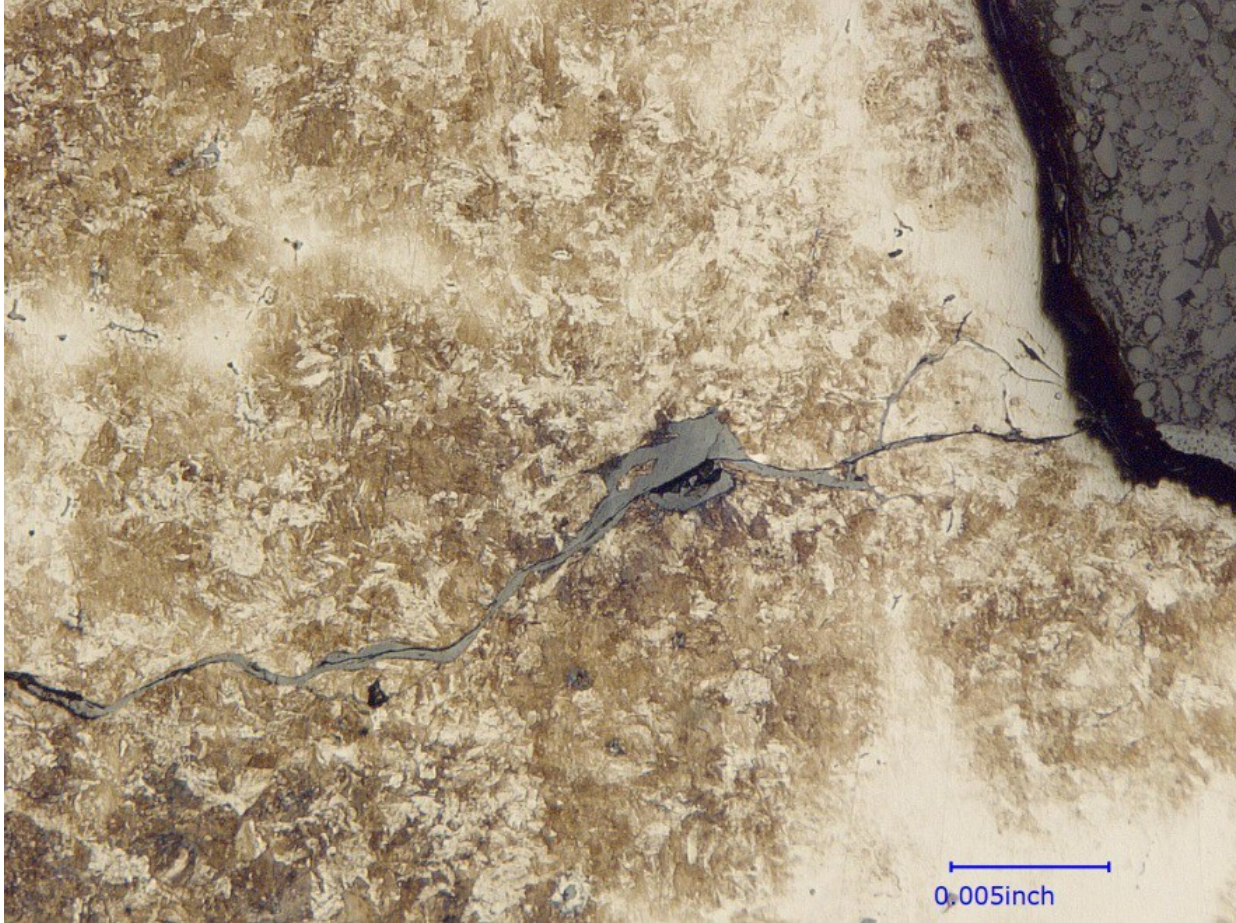
Figure A-33. Secondary Crack from BNSF6 VSR Face with Oxide, Original Magnification x200, Nital Etch
