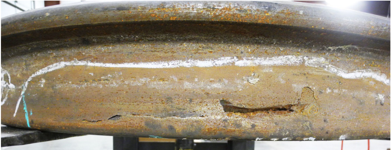
Figure A-10. Cracking on Tread of Wheel PR2
