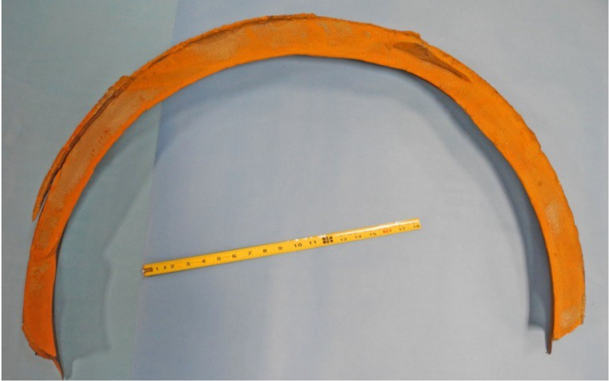
Figure A-42. Front Rim Section that Separated from Wheel CSX8
