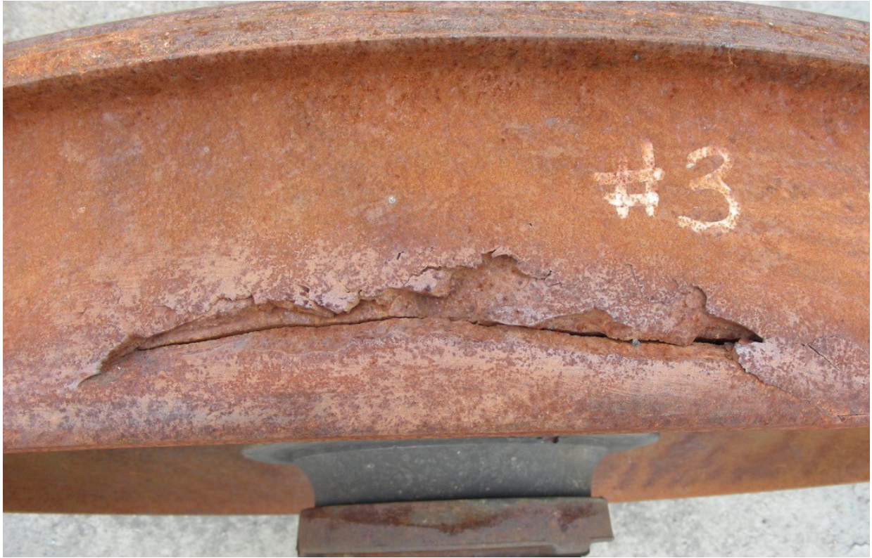
Figure A-35. VSR on Tread of Wheel BNSF7, BNSF Tread Photograph
