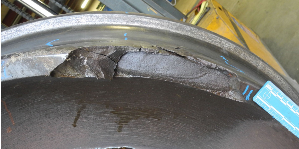
Figure A-52. Vertical Split Rim in Wheel UP9
