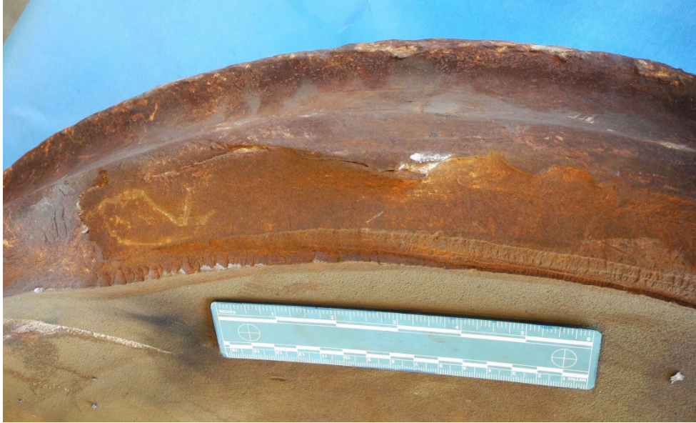
Figure A-16. VSR on Front Face of Wheel BNSF3
