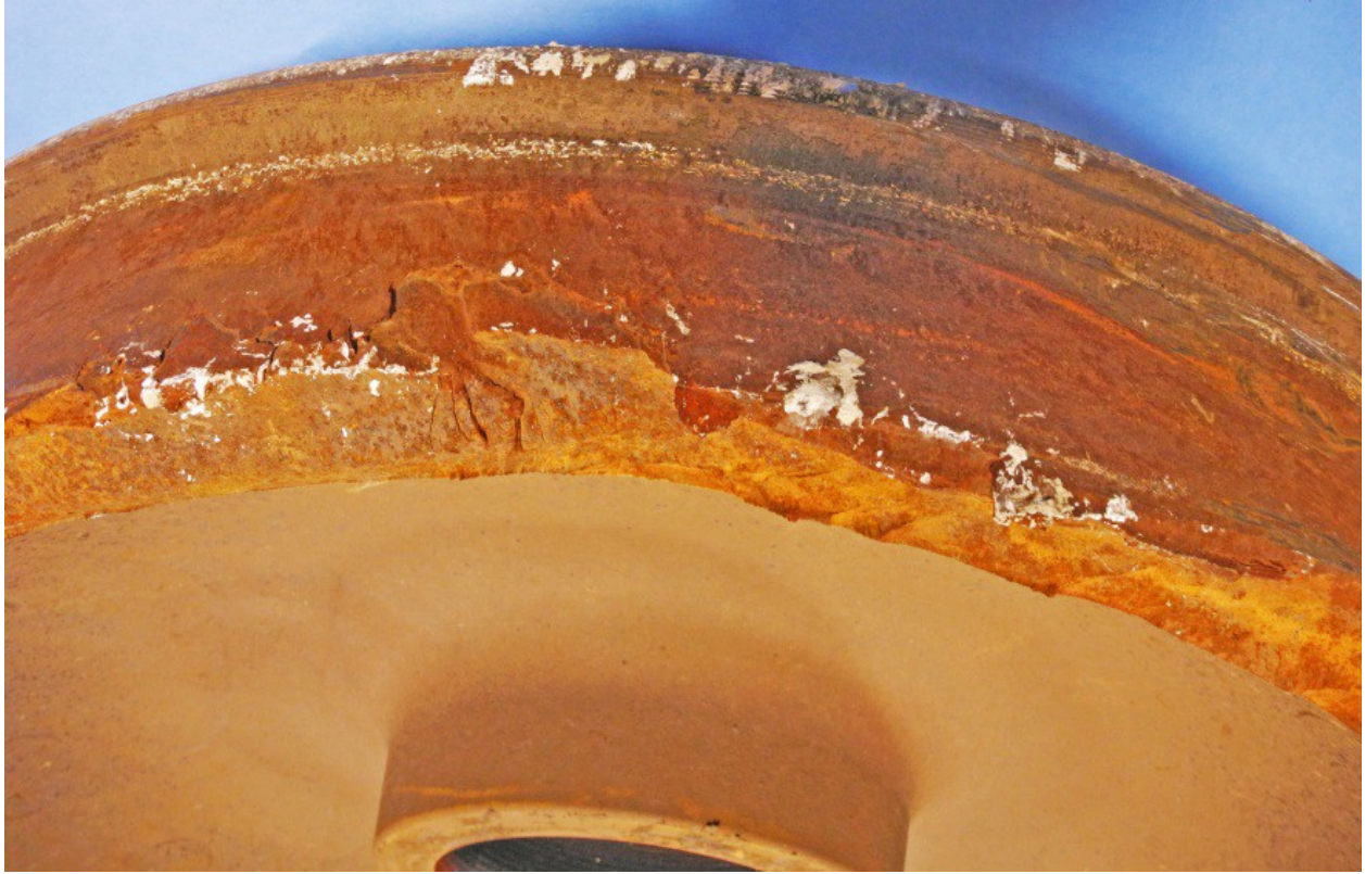
Figure A-30. Cracking on Tread of Wheel BNSF6
