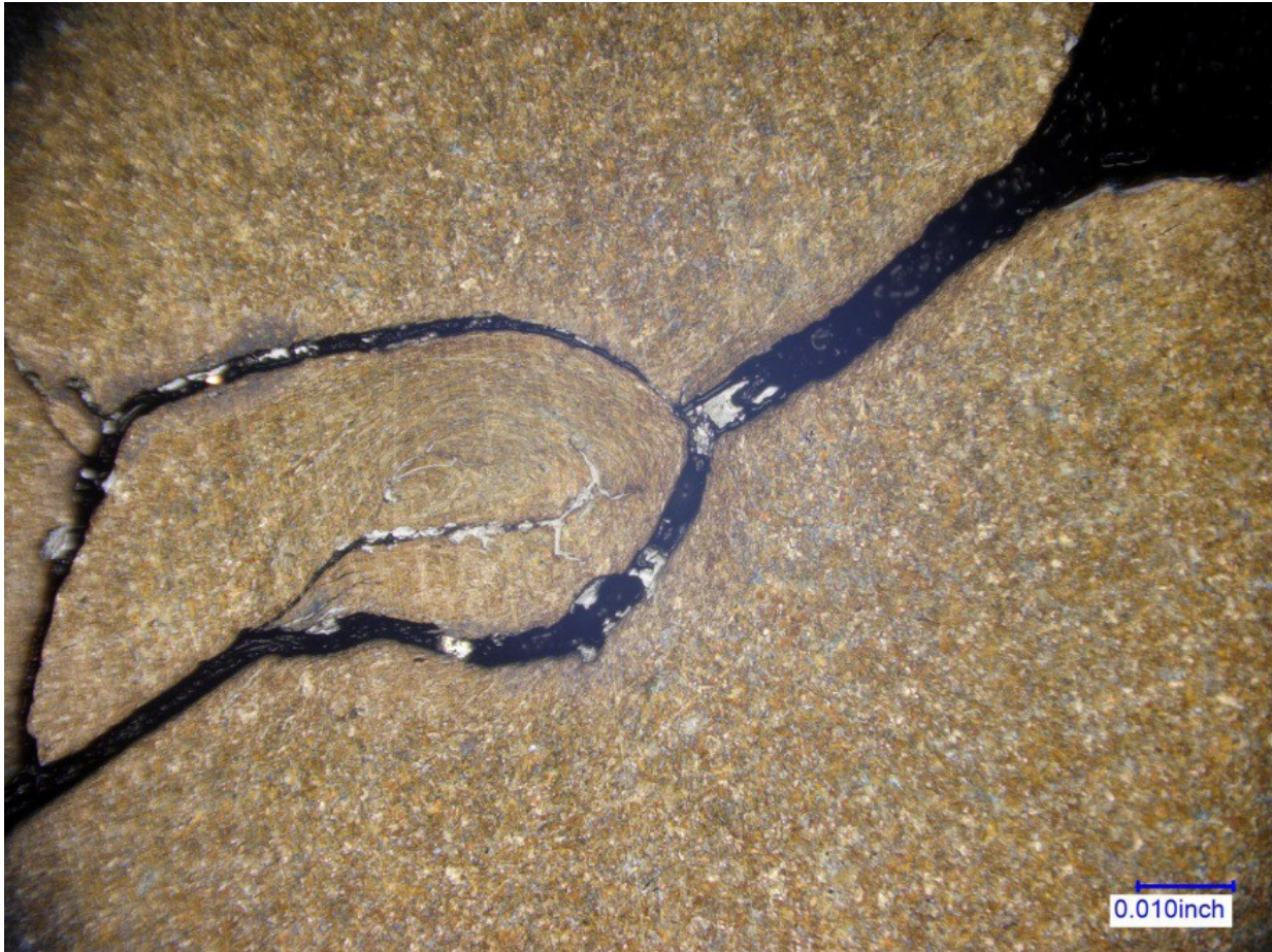
Figure A-39. Crack from Shelling in Wheel BNSF7, Original Magnification x100, Nital Etch
