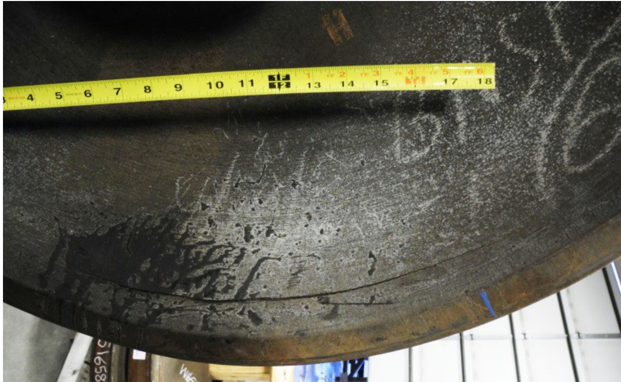
Figure A-23. VSR Crack in Wheel BNSF4 that Extended into Plate
