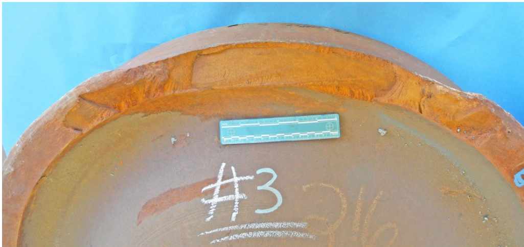
Figure A-17. VSR on Flange Side of Wheel BNSF3
