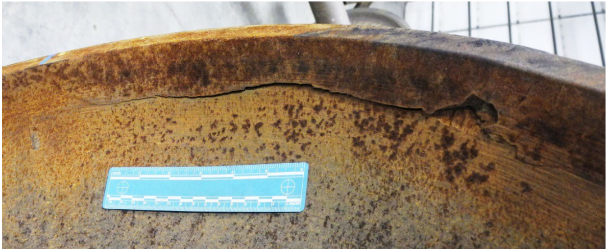
Figure A-36. Wheel BNSF7 VSR on Rim Plate Fillet
