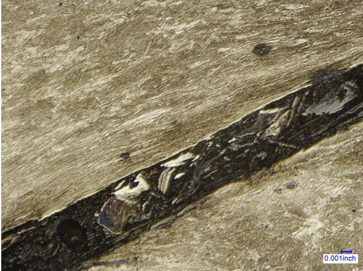
Figure A-15. Microstructure Above and Below PR2 Shell Crack, Original Magnification x1,000, Nital Etch
