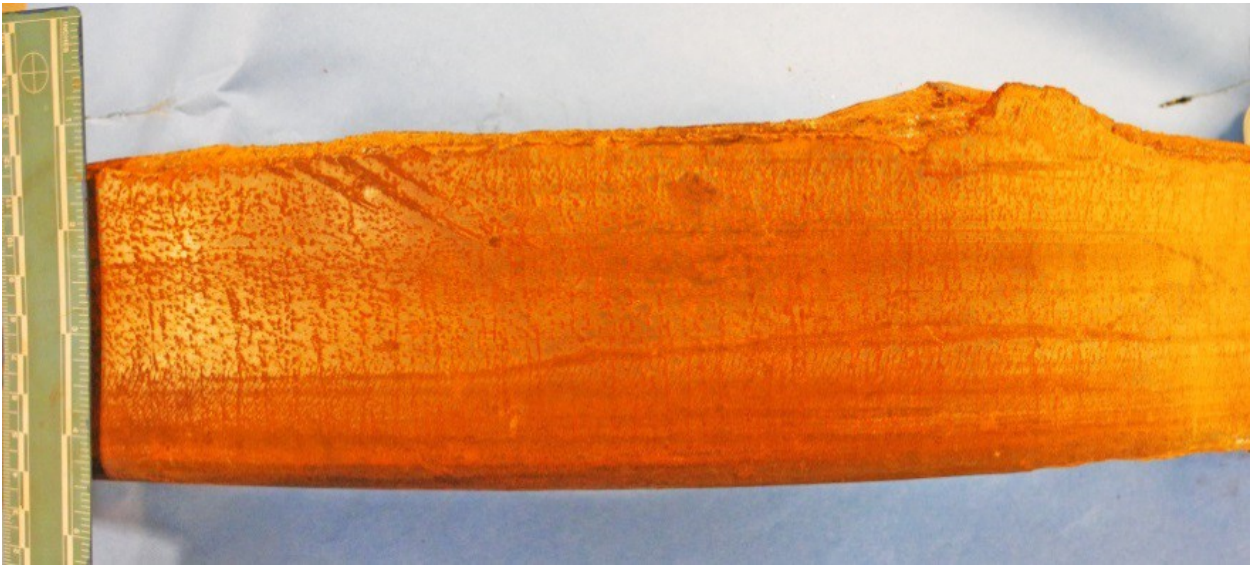
Figure A-43. Field Side Section of CSX8 Tread without Surface Shelling
