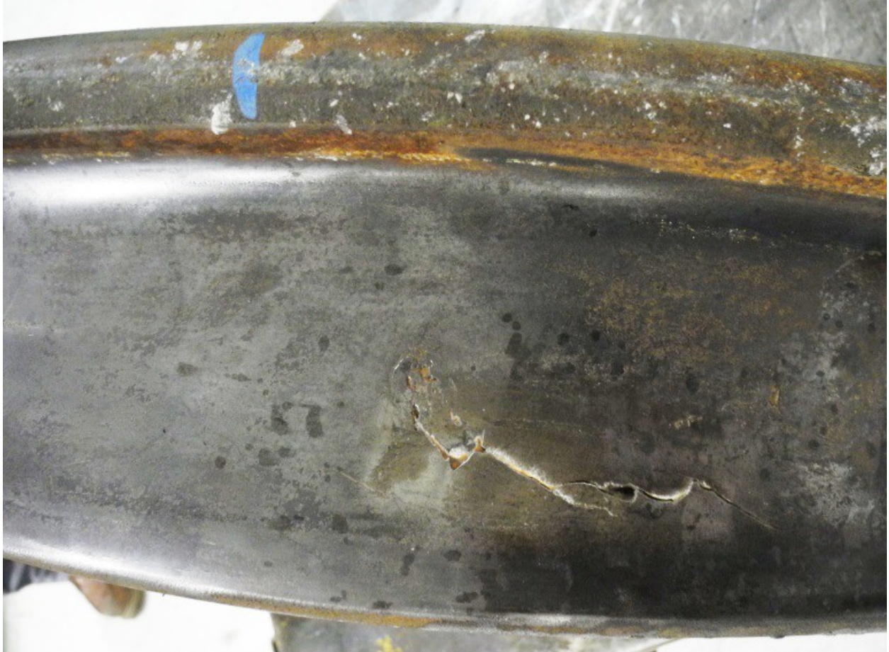
Figure A-22. Tread Crack in Wheel BNSF4
