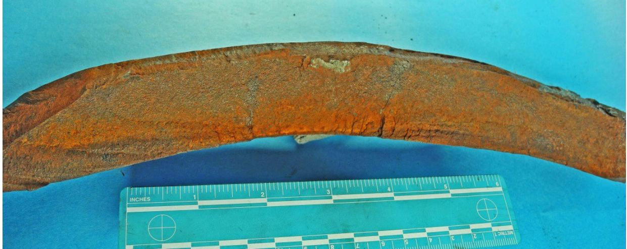
Figure A-37. Fracture Face of Wheel BNSF7 VSR
