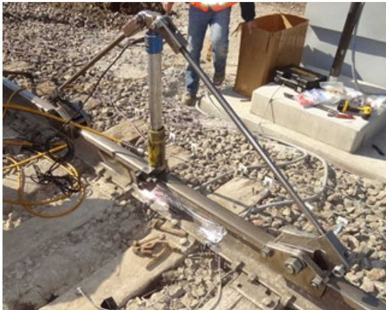
Figure 35. Strain Gauge Calibration Frame
