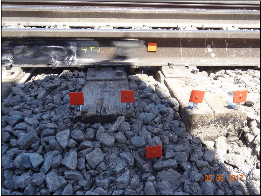
Figure 33. Targets Attached to Adjacent Cross-ties, Connecting Rail and Ground Stake
