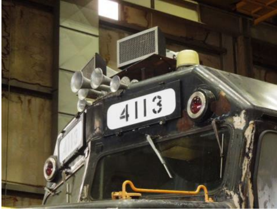
Figure 42. Nathan K5LA and \pm 15 Degree AWD Loudspeakers Mounted on the DOTX4113 Locomotive
