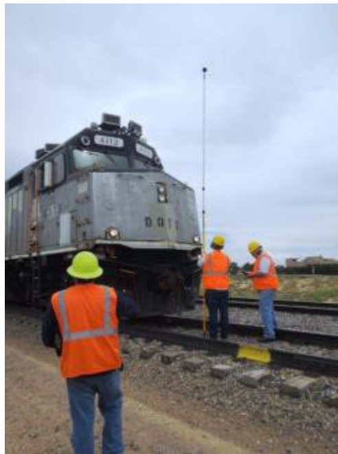
Figure 26. Sound Measurement with 15 Feet High Pole Right in Front of Locomotive
