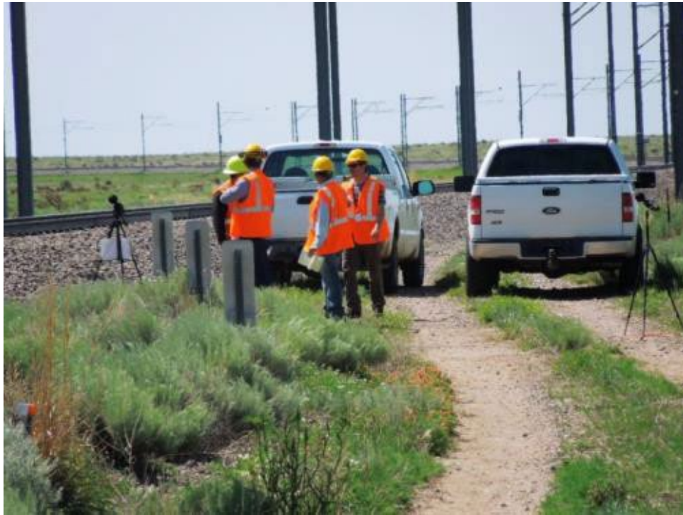
Figure 30. SLMs on Tripods Setup for Stationary Locomotive Horn/AWD Directivity Survey
