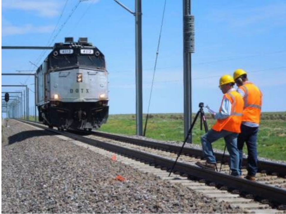
Figure 29. Static Locomotive Horn and AWD Directivity Measurement at 0 Degree Location
