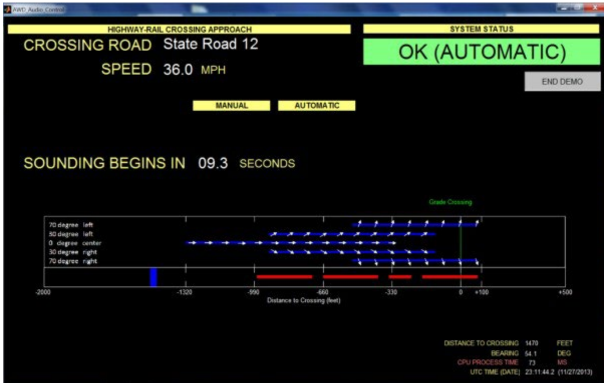
Figure 20. AWD Audio Control System Running (Demo Mode) – Approaching Sounding
