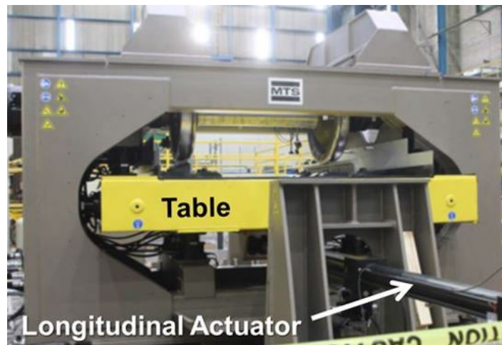
Figure 3. Reciprocating table activated by a longitudinal actuator
