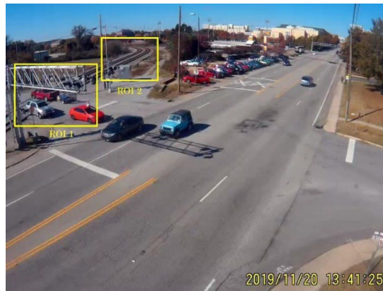
Figure 19. Two candidate ROIs for train passing time estimation
