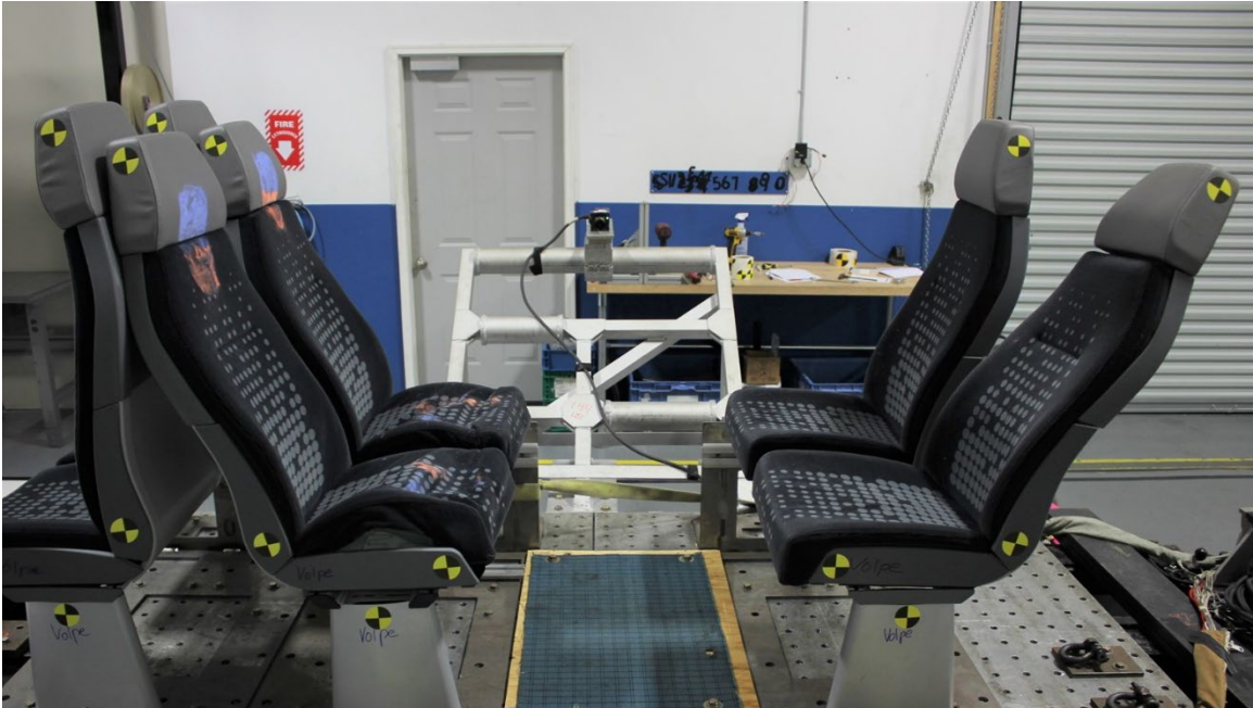
Figure 6: Test 1 Lateral Post-Test Photo
