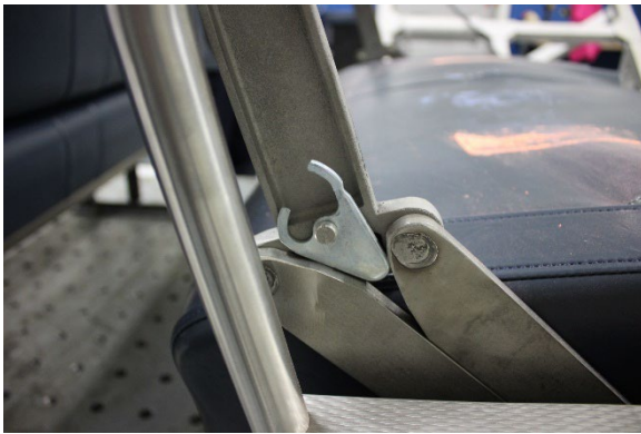
Figure 26: Test 2 Impact Seatback Rotational Lock
