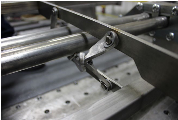
Figure 27: Test 2 Impact Seat Pan Structure
