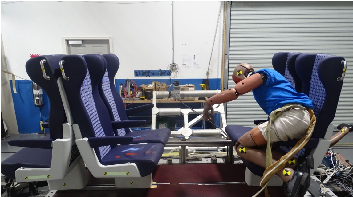
Figure 50: Test 4 Lateral Post-Test Photo
