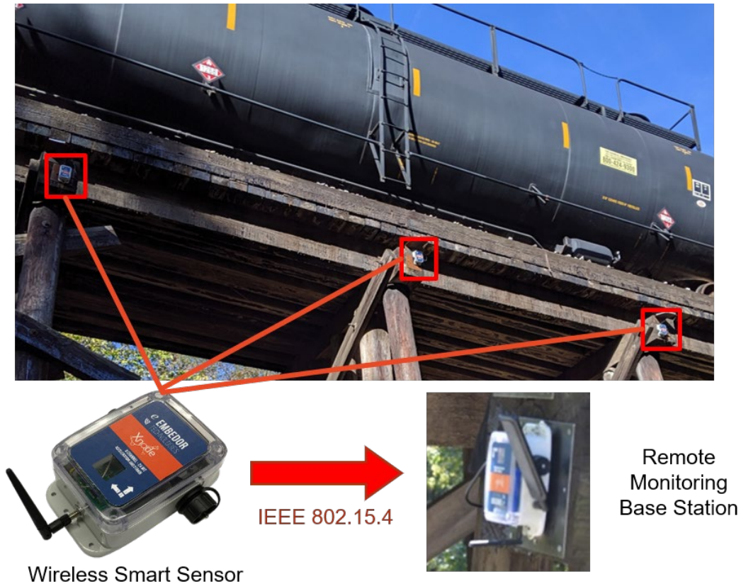
Figure 16: Bridge instrumentation plan (acceleration and displacement)
