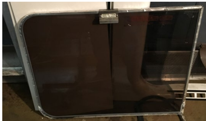
Figure 36. Window pane pulled into the car after the interior zip-strip was removed
