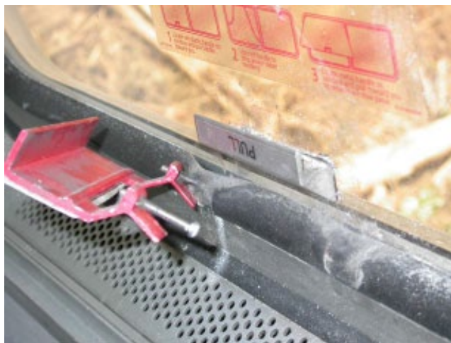
Figure 3. Example of malfunctioning emergency egress features from accident in Flora, MS
