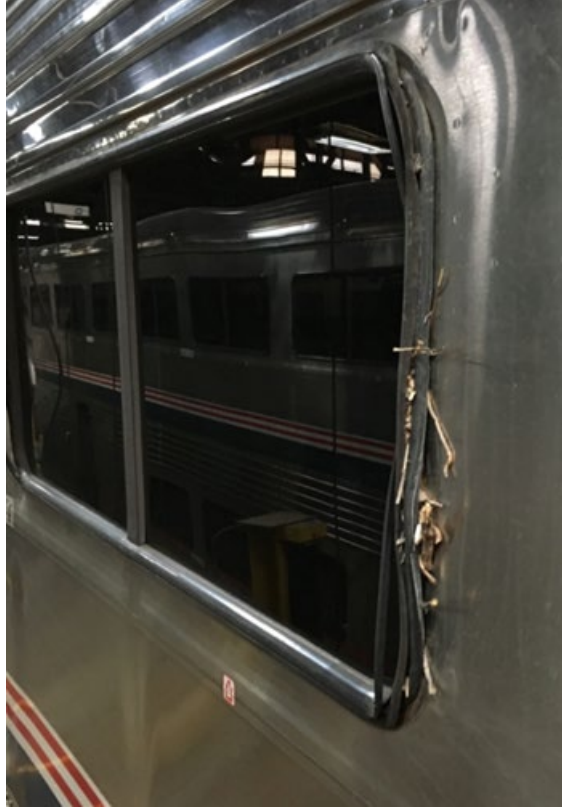
Figure 7. Debris collected from sliding along the ground, Cimarron, KS
