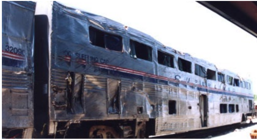
Figure 2. Result of derailment and rollover accident in Crescent City, FL
