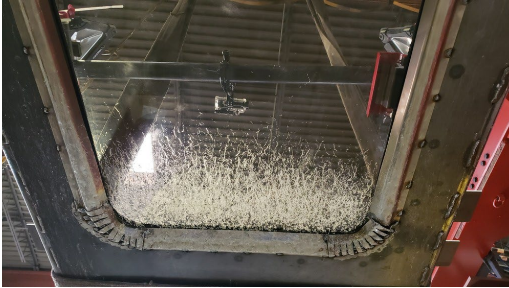
Figure 33. Drag test Specimen 8 – glazing intact after 86' of drag @ 950-lb load
