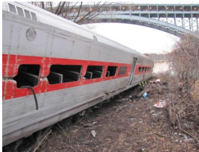
Figure 4. Result of derailment accident in Spuyten Duyvil, NY
