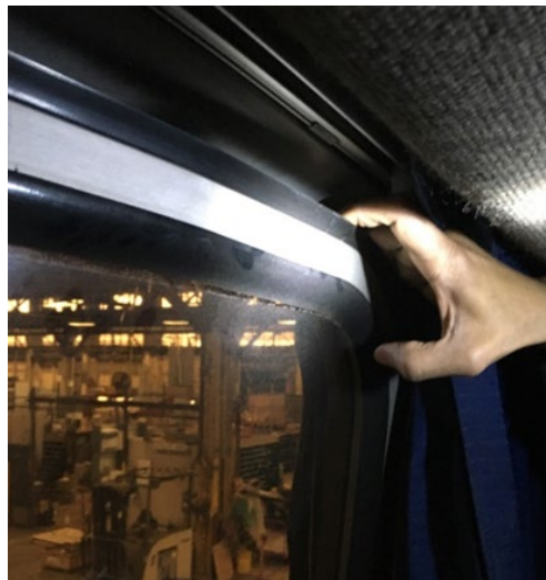
Figure 40. A demonstration of window and gasket system being pulled into the car
