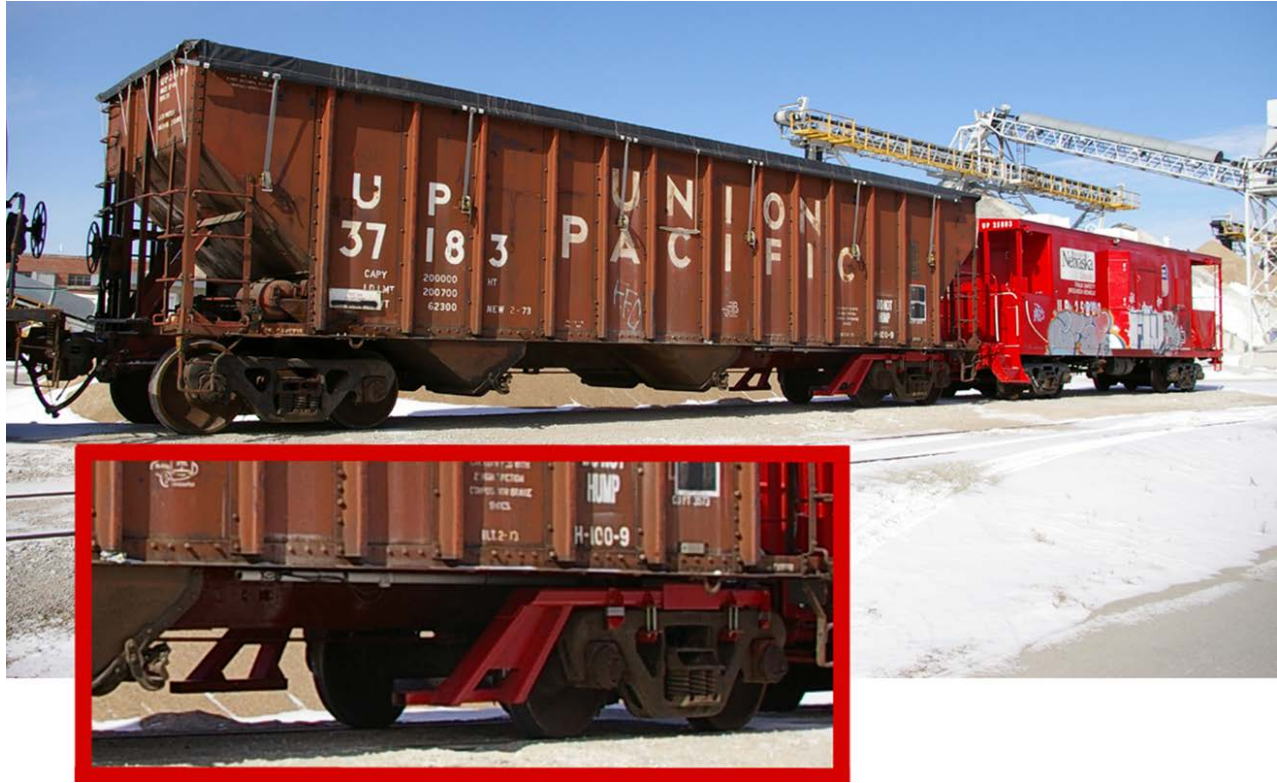
Figure 3-1 UNLX002 Hopper Car and Measurement System (Farritor and Fateh, 2013)
