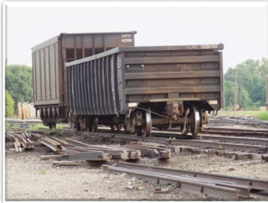
a) CN MRail Measurement Car
