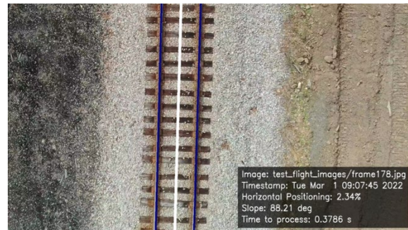
Figure 1: Onboard Track Centerline Detection
