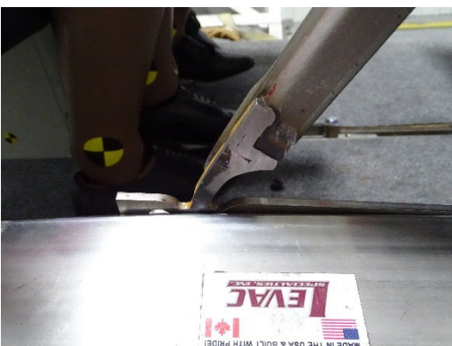
Figure 37. Test 2BD Workstation Table Rear Wall Mount
