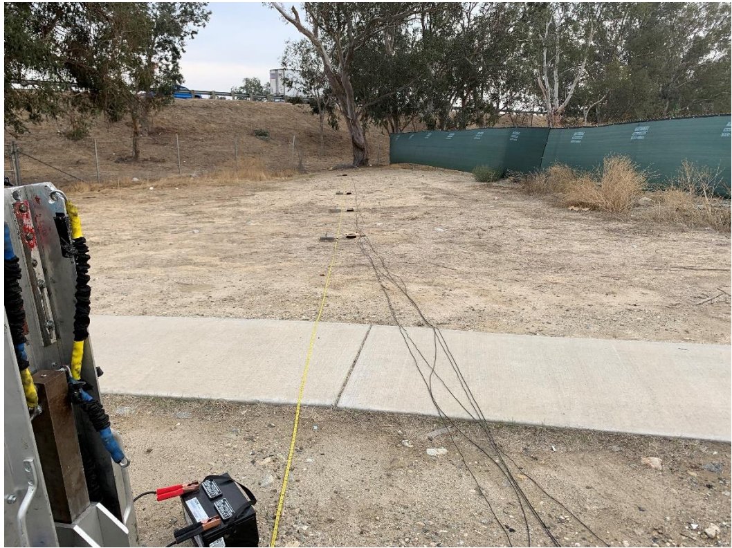
Figure B-1: Transfer Mobility Measurement Site V-1 7540 Crawford Place
