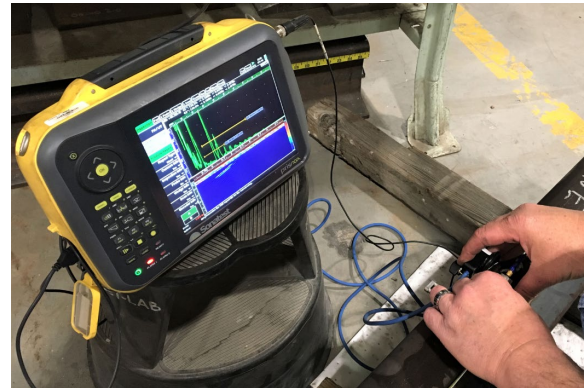
Figure 3. Hand-held PAUT rail flow characterization
