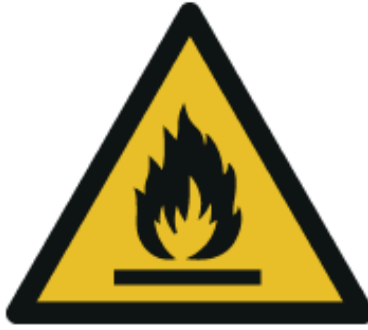
Figure 11: Flammability/Naked Flames Warning (European Standard, 2013)
