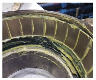
Figure 9. Bearing Running Surface After Second Test
