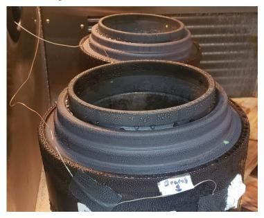
Figure 4. Bearings in Environmental Chamber
