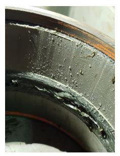
Figure 1. Bearing Cup Running Surface with Water Ingress
