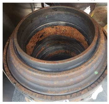
**Figure 5. Corrosion on Bearing Surfaces**
