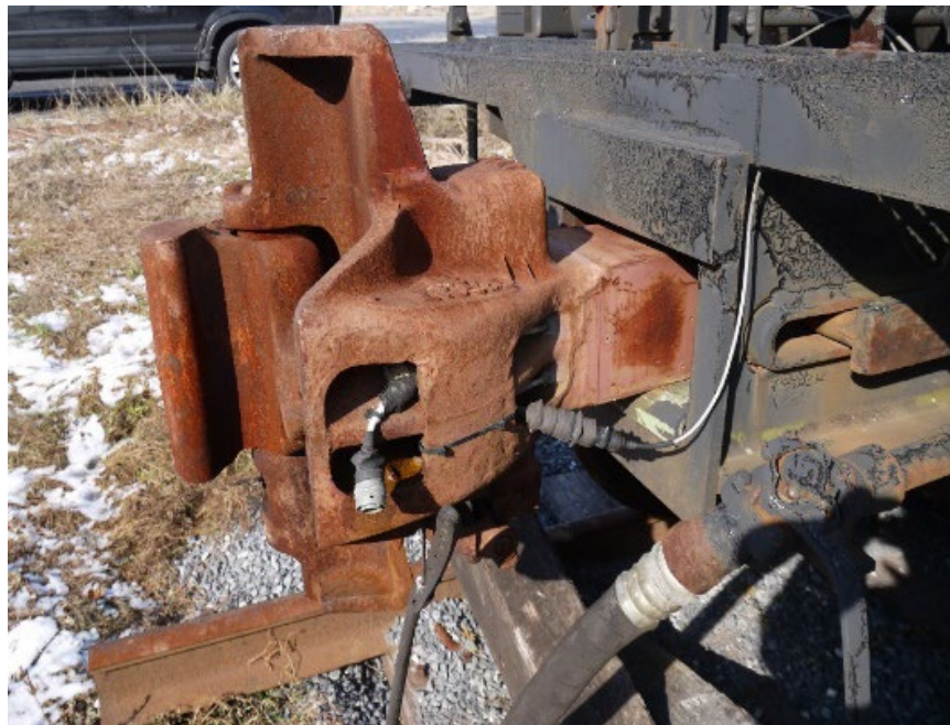
Figure 6. Instrumented Coupler for Measuring Longitudinal Coupler Forces
