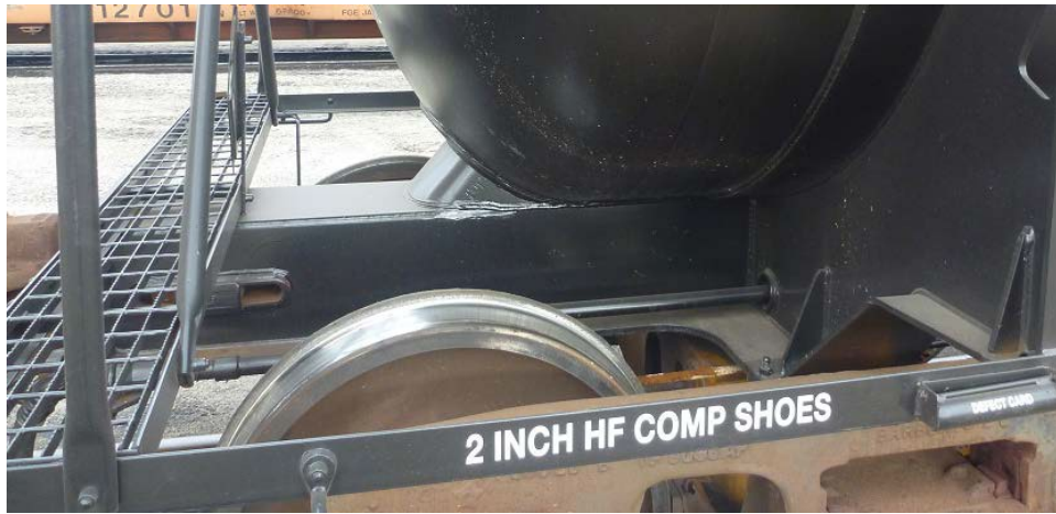
Figure 4. Detail View of the Stub Sill and Head Brace Attached to the Tank of the Instrumented Tank Car
