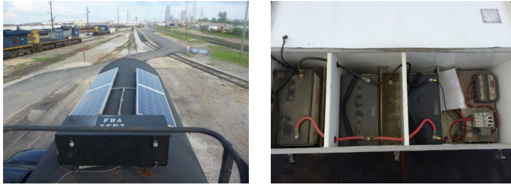
Figure 8. Solar Panel and Battery Box on Top of Instrumented Tank Car
