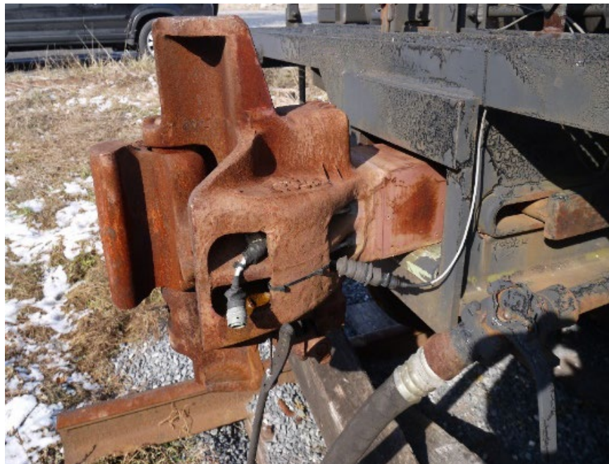
Figure 6. Instrumented Coupler for Measuring Longitudinal Coupler Forces
