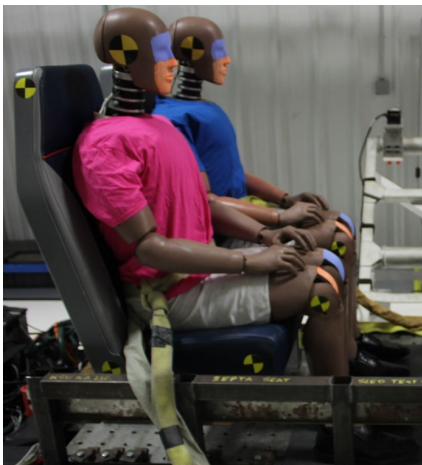
Figure 1. Pre-test Photo of APTA Seat Standard Test with the Commuter Rail 2-passenger Seat
