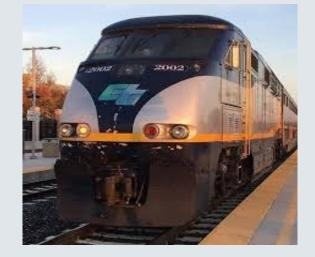
F59PHI (EMD) Year introduced: 1991 / 2001 Emission standard: Tier 2 Power: ~2200 kW
