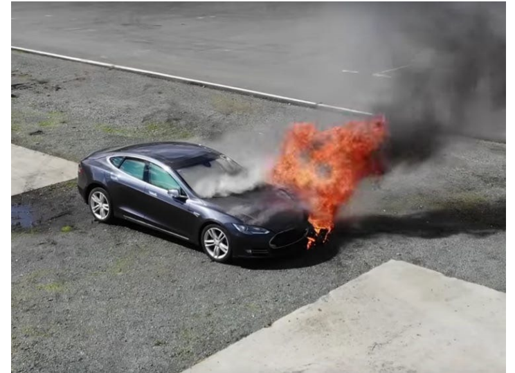
Tesla NMC battery fire [Source: www.businessinsider.com ]
