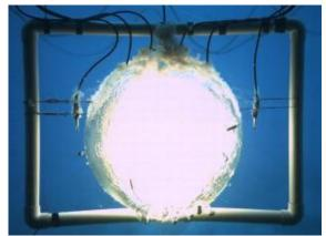
Both lithium and lithium-ion battery failures can result in unwanted, uncontrolled, energy release
