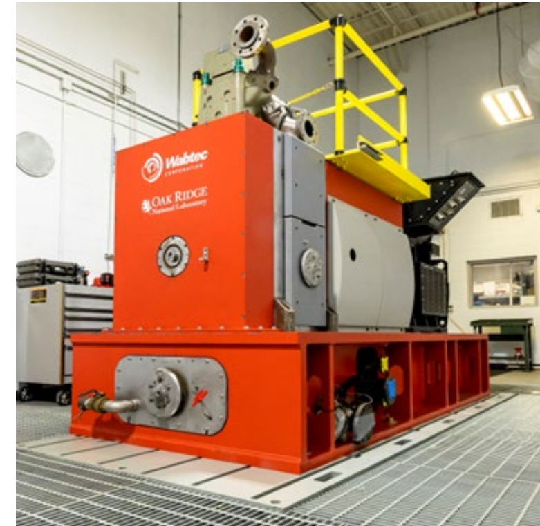
Wabtec single-cylinder locomotive research engine installed at NTRC
